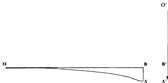
Figure 1. The path of a horizontally emitted ray of light and that of a free-falling cabin in vertically directed homogeneous gravitational field.
