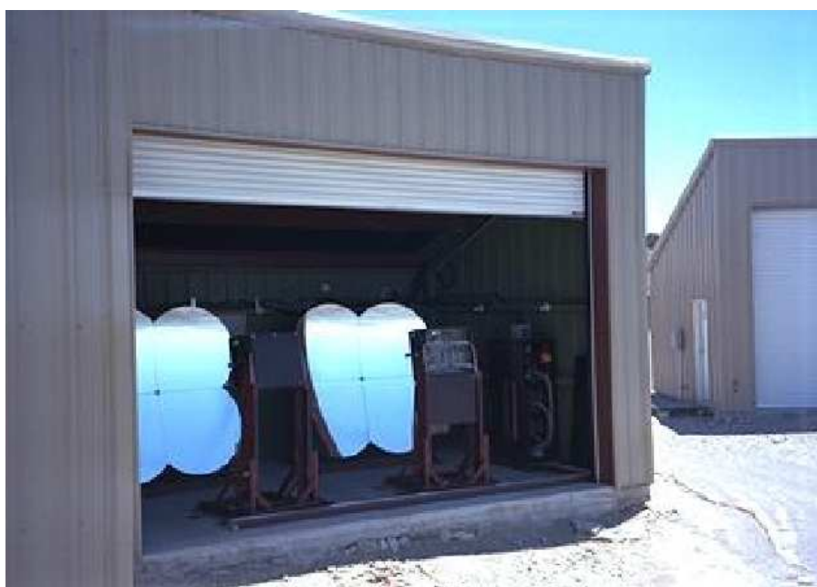
Figure 2.3: Detector housings of the HiRes experiment. Two detector units (mirror and PMT cluster) can fit in one building.
