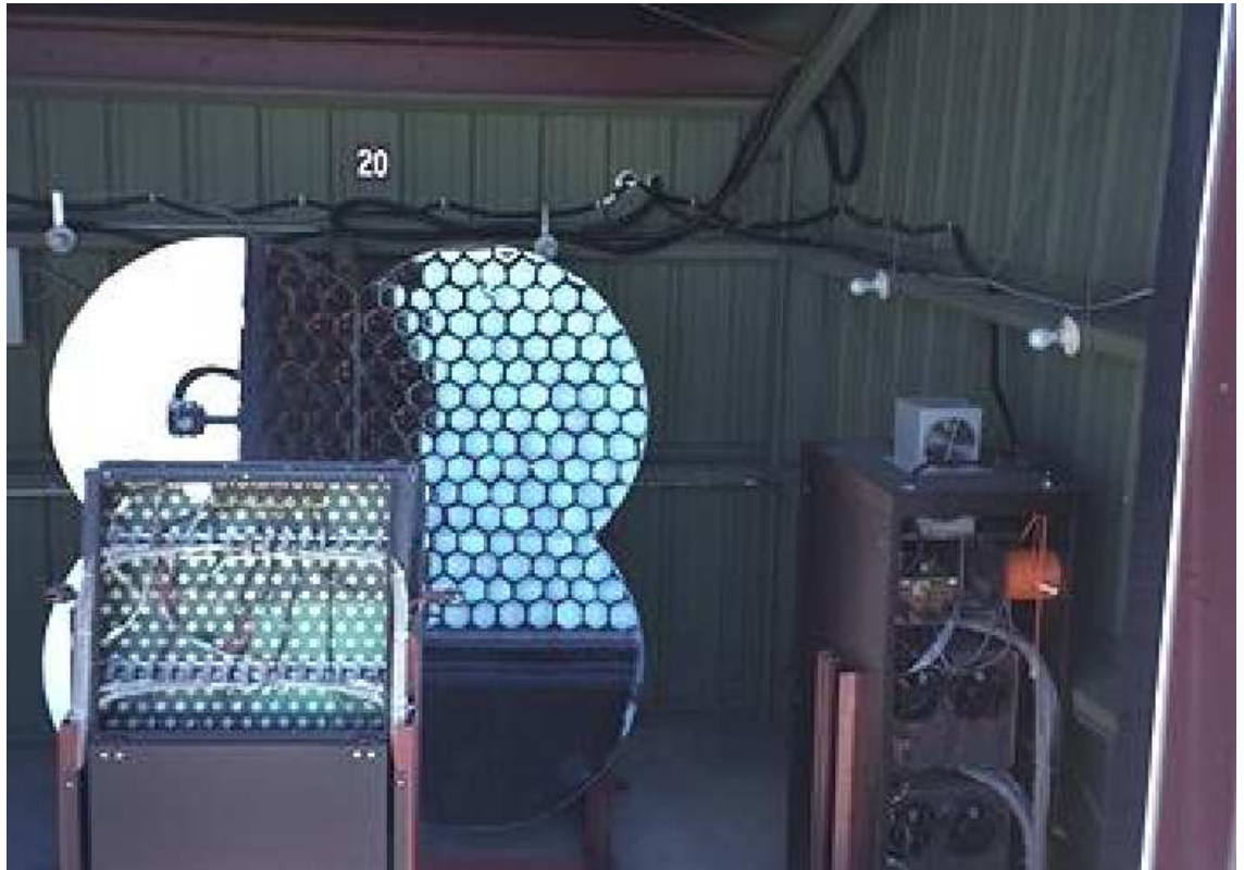
Figure 2.7: HiRes mirror unit. The UV filter has been removed, so that the hexagonal pattern of the phototubes can be seen as a reflection in the mirror.
