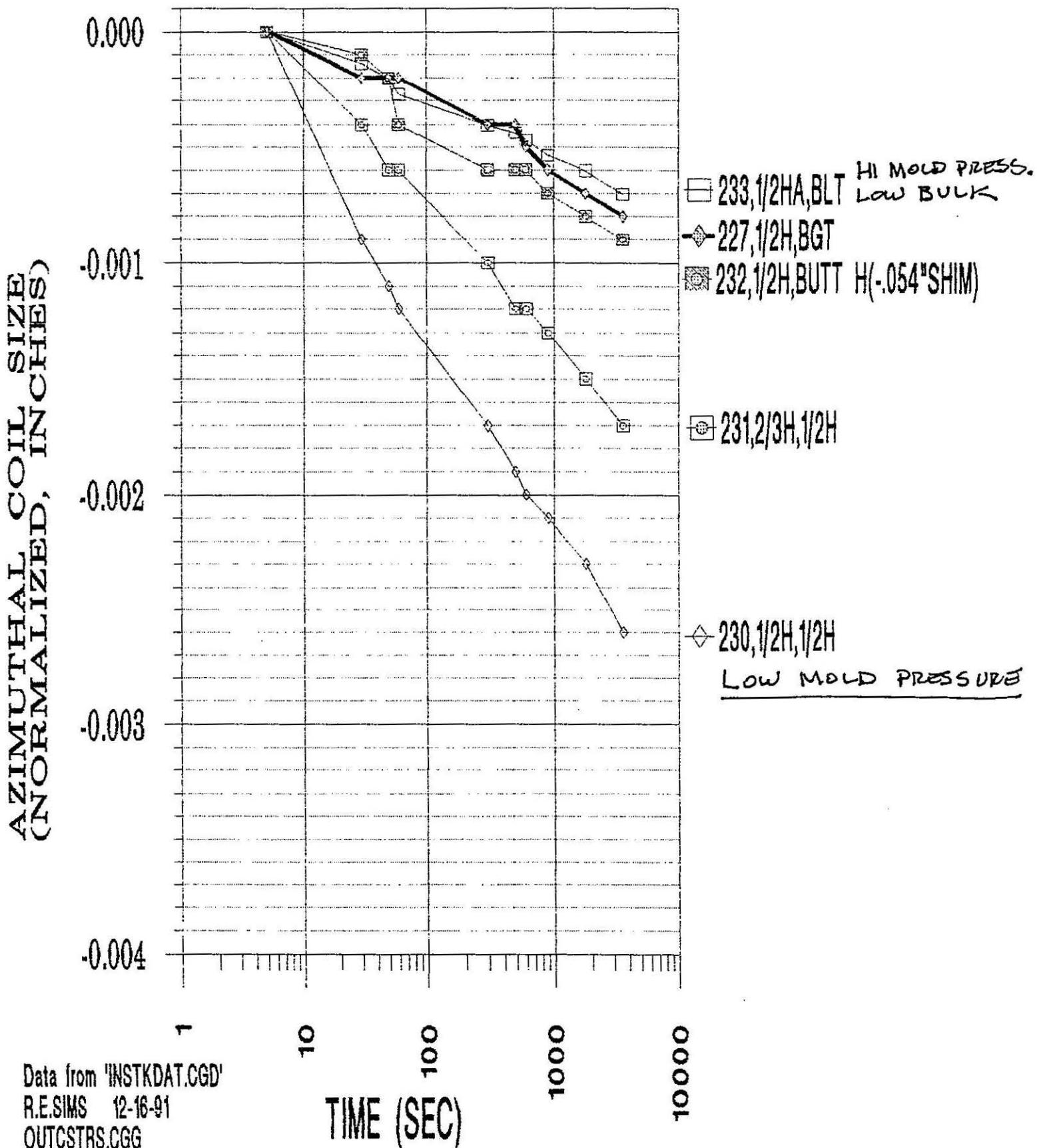
TEN STACK STRESS RELAXATION WITH 12 KPSI FOR ONE HOUR (SSC 50mm INNER CABLE)
