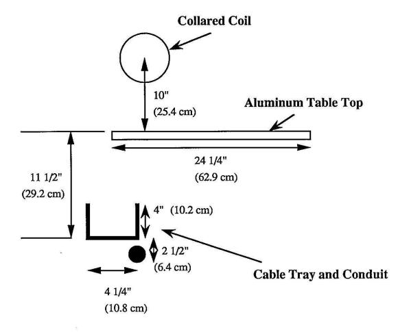
Figure 1. Industrial Center Building Aluminum Table Showing Table, Magnet, and Cable Tray Relative Locations During Test
