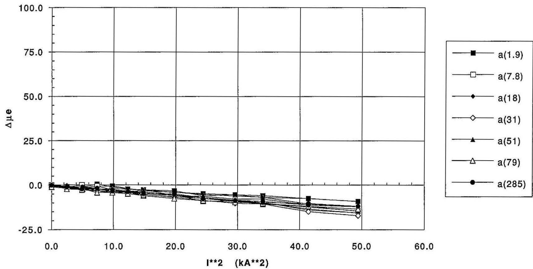
**DCA313 Shell Strain Gauges at z = 1297 mm**
