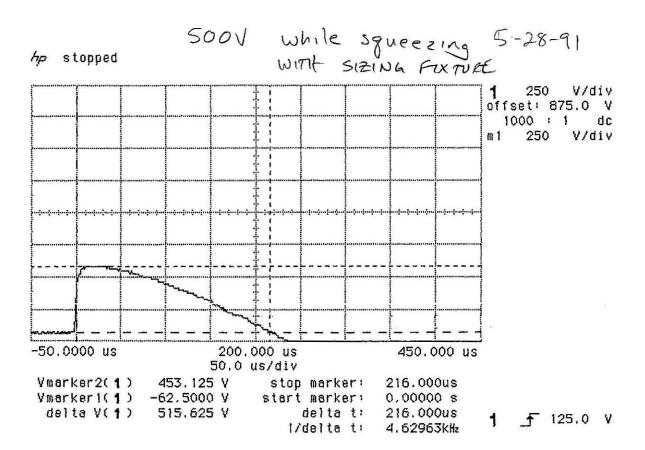
1000 V while squeezing with sizing fixture 5-28-91 hp stopped 1 250 V/div offset: 875.0 V 1000 : 1 dc ? 250 V/div m2 -50.0000 us 200.000 us 450.000 us 50.0 us/div Vmarker2(1) 453.125 V stop marker: 216,000us start marker: delta t: Vmarker1(1) -62,5000 V 0,00000 s del ta V(1) 515.625 V delta t: 216.000us 1 \_f 125.0 ¥ 1/delta t: 4,62963kHz
