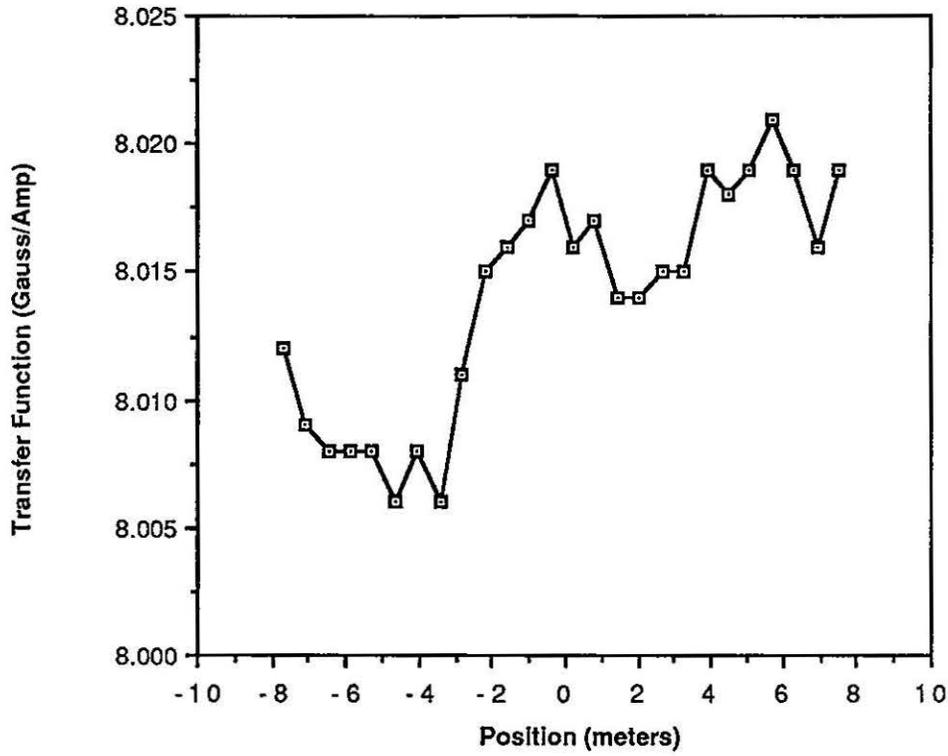
Figure 1d. DC0303 Transfer Function
