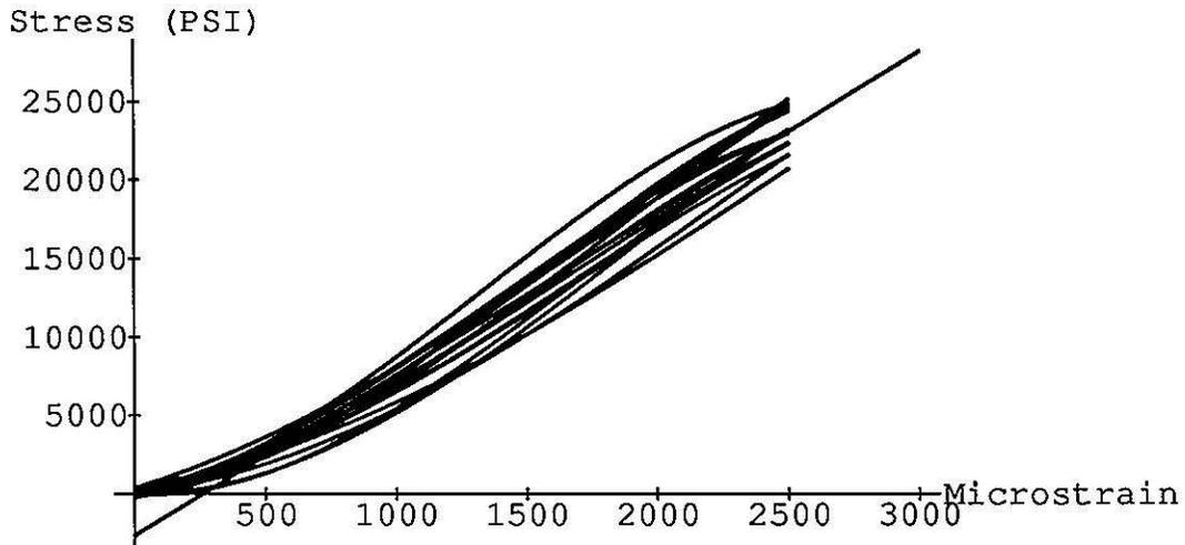
FNL gages calibrated at FNL at about 4.2°K. The line shown is the best linear fit to these curves over the range of 200 to 2500 microstrain. It has the form  $-2681+10.3x$ .
