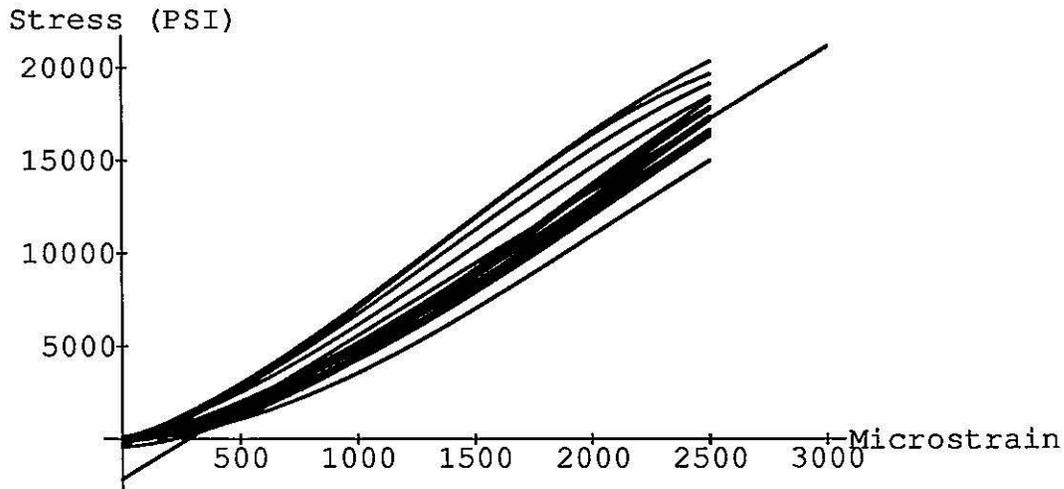
FNL gages calibrated at FNL at about 300°K. The line shown is the best linear fit to these curves over the range of 200 to 2500 microstrain. It has the form  $-2162+7.76x$ .
