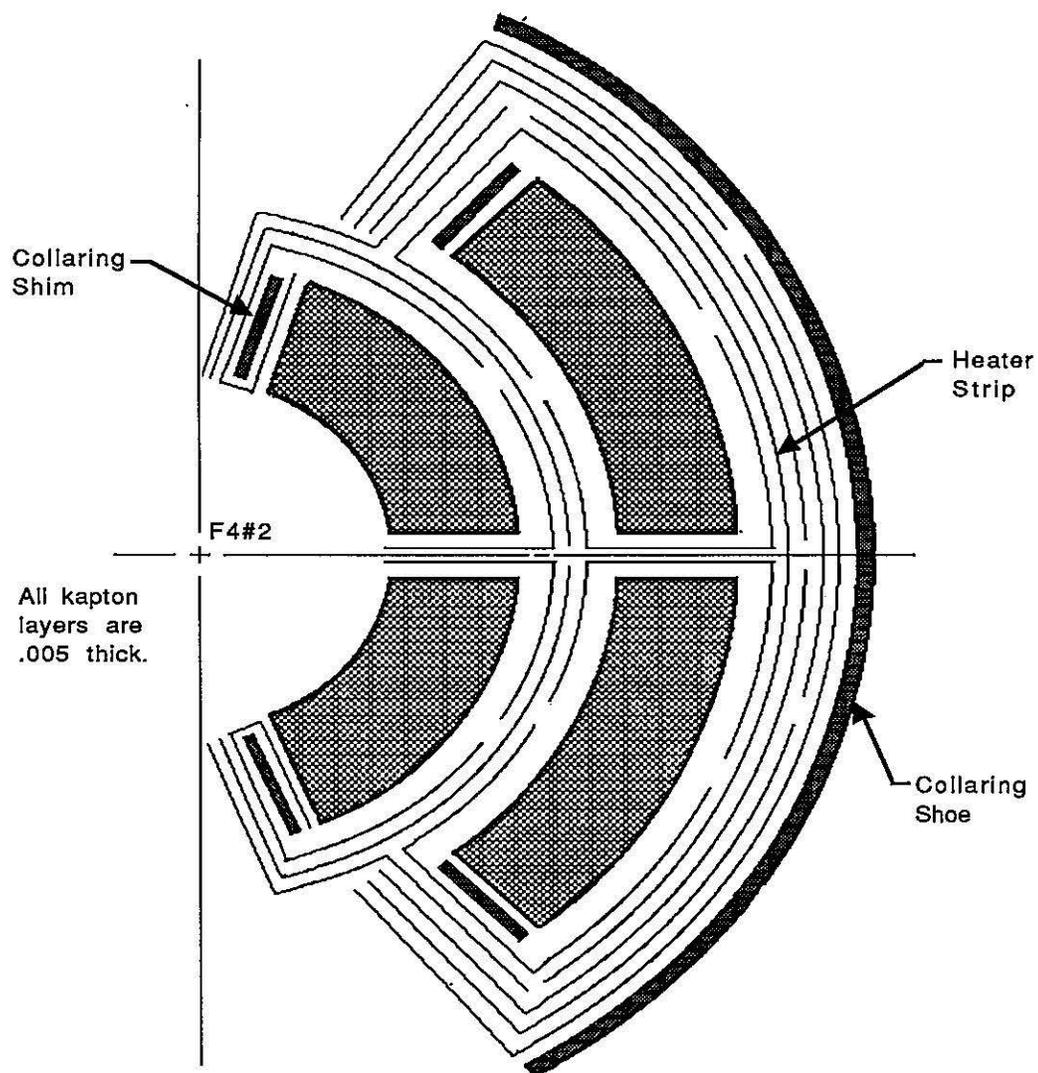
The insulation scheme in Figure 3 is an attempt to; 1.) retain the inner coil collaring shim while still allowing helium flow between the bore area and the collars and 2.) retain the outer coil collaring shim without eliminating the collaring shoe.
