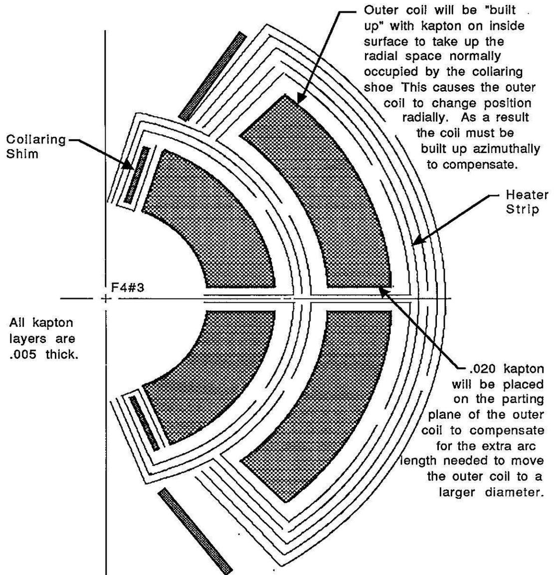
After these sections have been collared they will be potted and cut into cookies. They will be examined to determine what the coil insulation scheme will be for the rest of the F series magnets.
