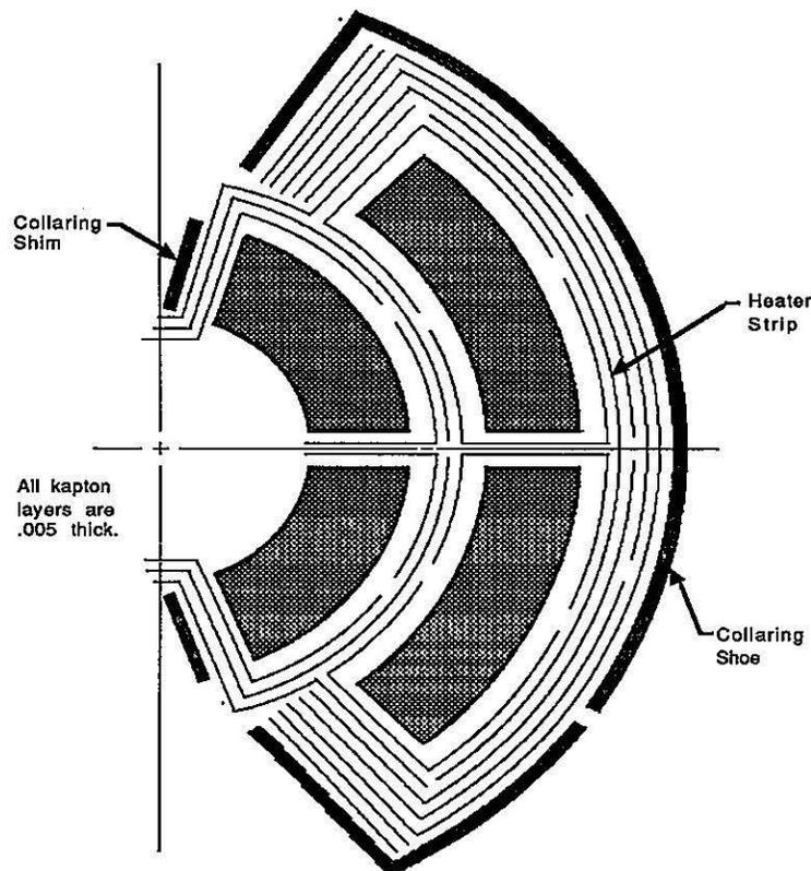
The inner coil kapton insulation was connected at the pole. This provided a restraint to prevent the inner coil collaring shim from moving inward. The brass collaring shoe and the outer coil collaring shim were connected. They were made of one piece, with a preformed corner to prevent the shim from being driven into the inner coil.
