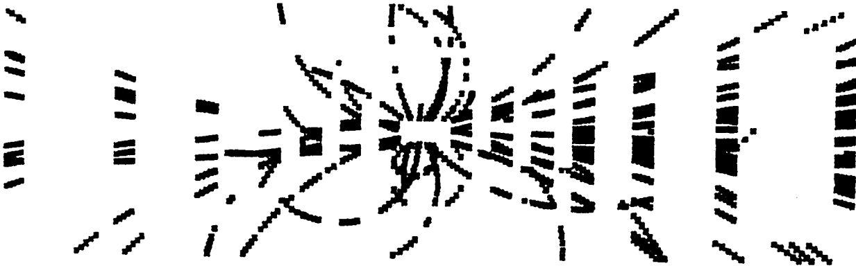
Figure 18: A typical SSC event from the b\bar{b} two-jet process, showing all minivectors in the straw tracking system.
