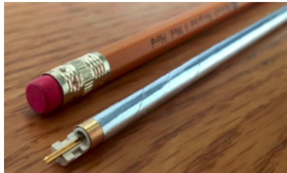
Figure 3.6: One of the Mu2e straw tube (compared to a pencil) [81].
