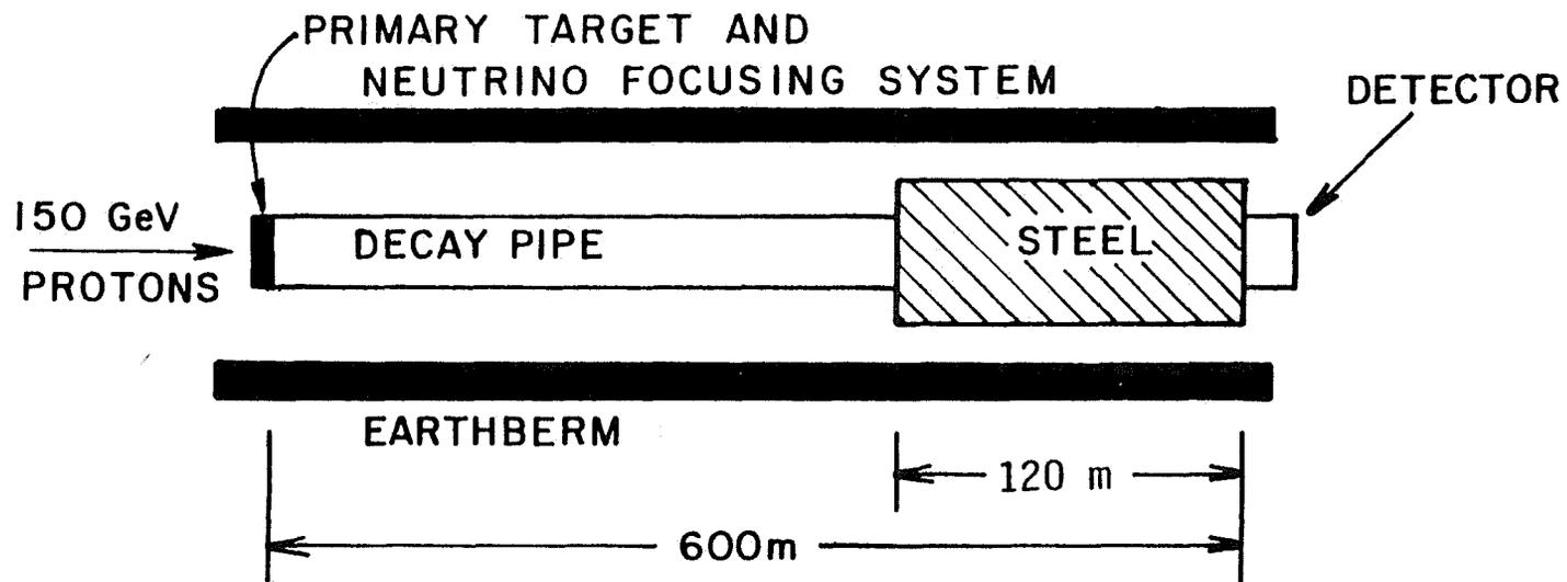
**FIGURE 4:** Layout of proposed neutrino beam line showing the location of the proposed oscillation experiment.
