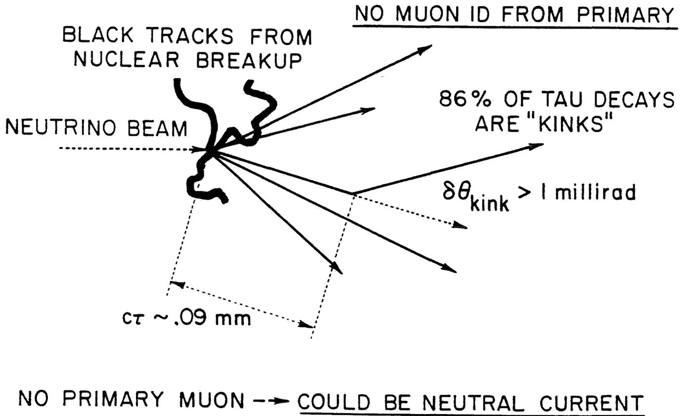
**FIGURE 3:** Schematic picture of a  $\nu_\tau$  interaction. Note the heavily-ionizing tracks from nuclear breakup, the absence of an identified muon from the interaction vertex and a short decay-length "kink" with a large  $P_T$ .
