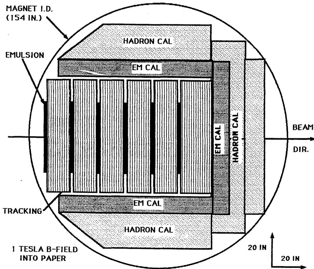
SCINTILLATOR COUNTERS DOWNSTREAM OF ALL EMULSION MODULES AND IN ALL CALORIMETERS NOT SHOWN. MOST MUONS IDENTIFIED BY RANGE AND P.H. IN THE CALORIMETERS. RANGE WALL DOWNSTREAM OF COILS FOR CENTRAL HIGH-ENERGY MUONS NOT SHOWN.
