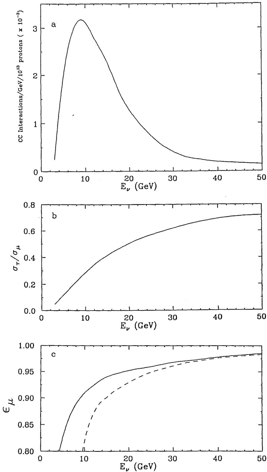
**FIGURE 5:** a) Charged-current event rate for the 150 GeV high-flux neutrino beam. The calculation assumes a 400 meter decay pipe, 120 meter shield and a double-horn focussing system.
