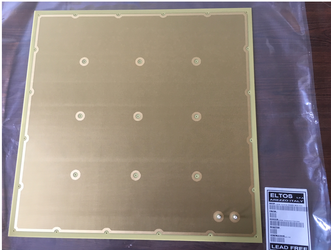
Figure 2.8: Picture of a LEM module used for ProtoDUNE-DP
