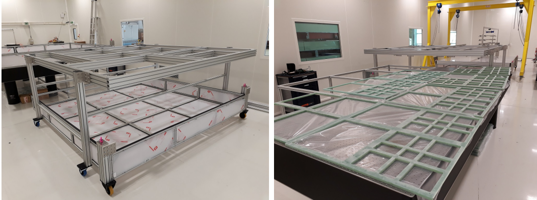
Figure 2.19: Elements for assembly of ProtoDUNE-DP CRP in clean room 185 at CERN: assembly structure and G10 subframes being prepared.
