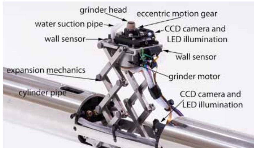
Figure 2.5 Local grinding tool with an expandable motor stage installed in a 50-mm-diameter cylindrical housing.
