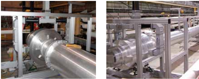
Figure 2.23 KCS R&D hardware. Left: coaxial tap-off fed through a waveguide T and connected through a taper to the 0.480-m diameter circular waveguide. Right: a four-section 10-m run of the KCS main waveguide.
