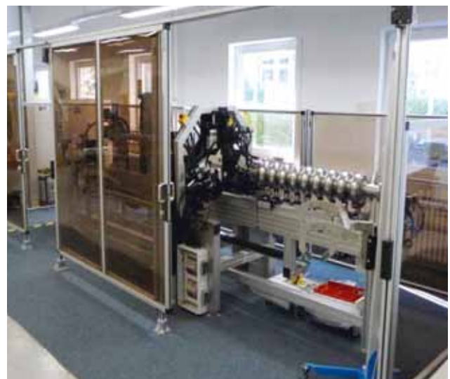
Figure 2.12 Left: tool for room temperature RF measurement of half cells. Right: tool for field flatness tuning of completed cavities.
