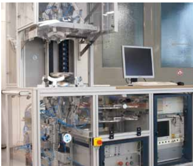
Figure 2.12 Left: tool for room temperature RF measurement of half cells. Right: tool for field flatness tuning of completed cavities.
