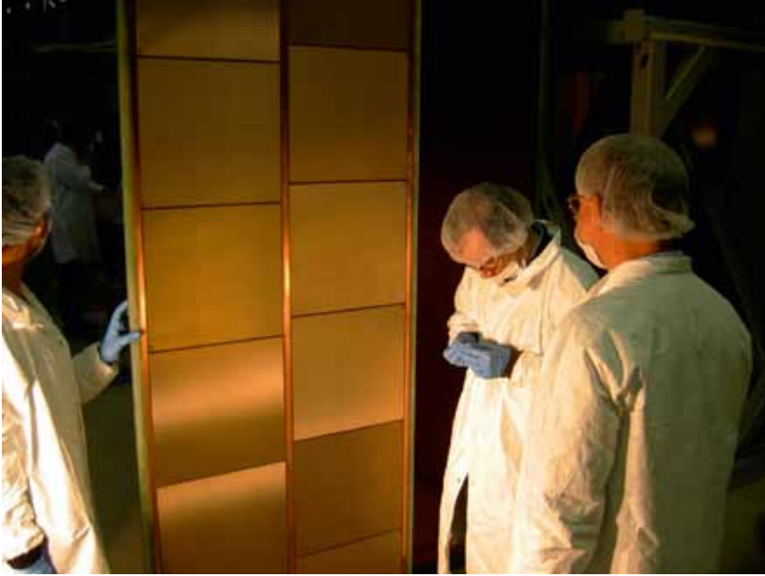
Figure 5.5 Micromegas readout plane for the near detector of the T2K experiment, the development of which fully originated out of R&D carried out for the ILC. Image: T2K Collaboration
