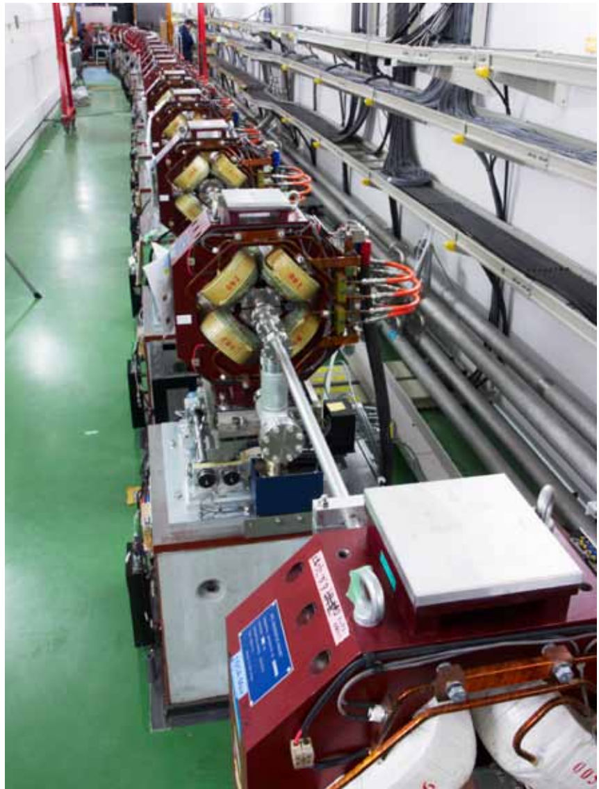
Figure 3.11 View looking downstream along the final focus section of the ATF2 beamline.
