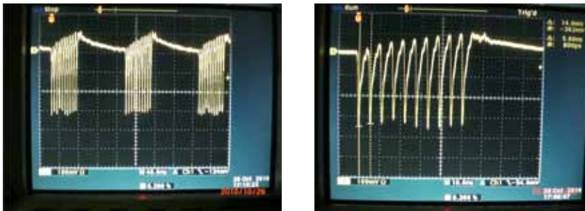
Figure 3.28 ATF damping ring. Top: three trains of ten bunches with 5-ns spacing (right image is a close-up of waveforms seen in the left image). Bottom: 30 bunches extracted with 308-ns spacing.
