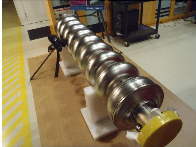
Figure 1. Superconducting niobium radio frequency cavity.
