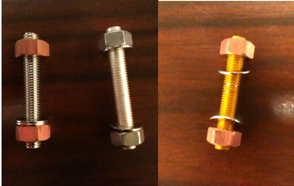
Figure 11. Steel, silver, and TiN studs.
