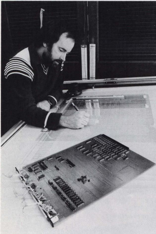
Larry Bays works on the design of a printed circuit.
