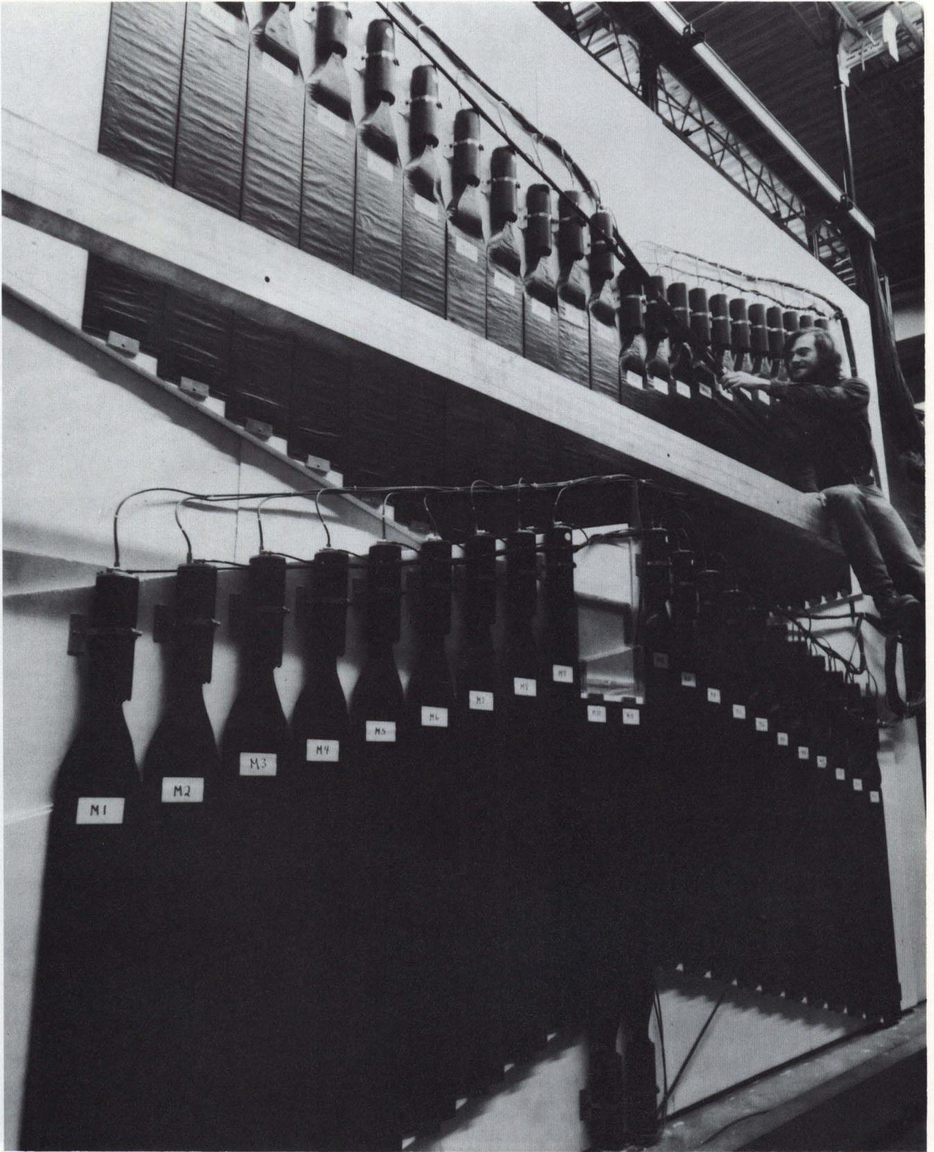
Pat Lukens (Illinois) installs detectors in E-673 in the Muon Laboratory.
