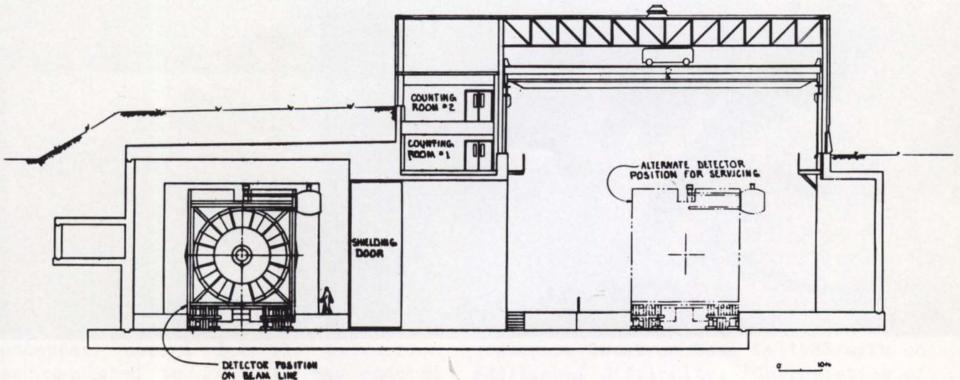
An end view of the entire facility. The beam tunnel and collision area are at the left and the Assembly Area at the right.
