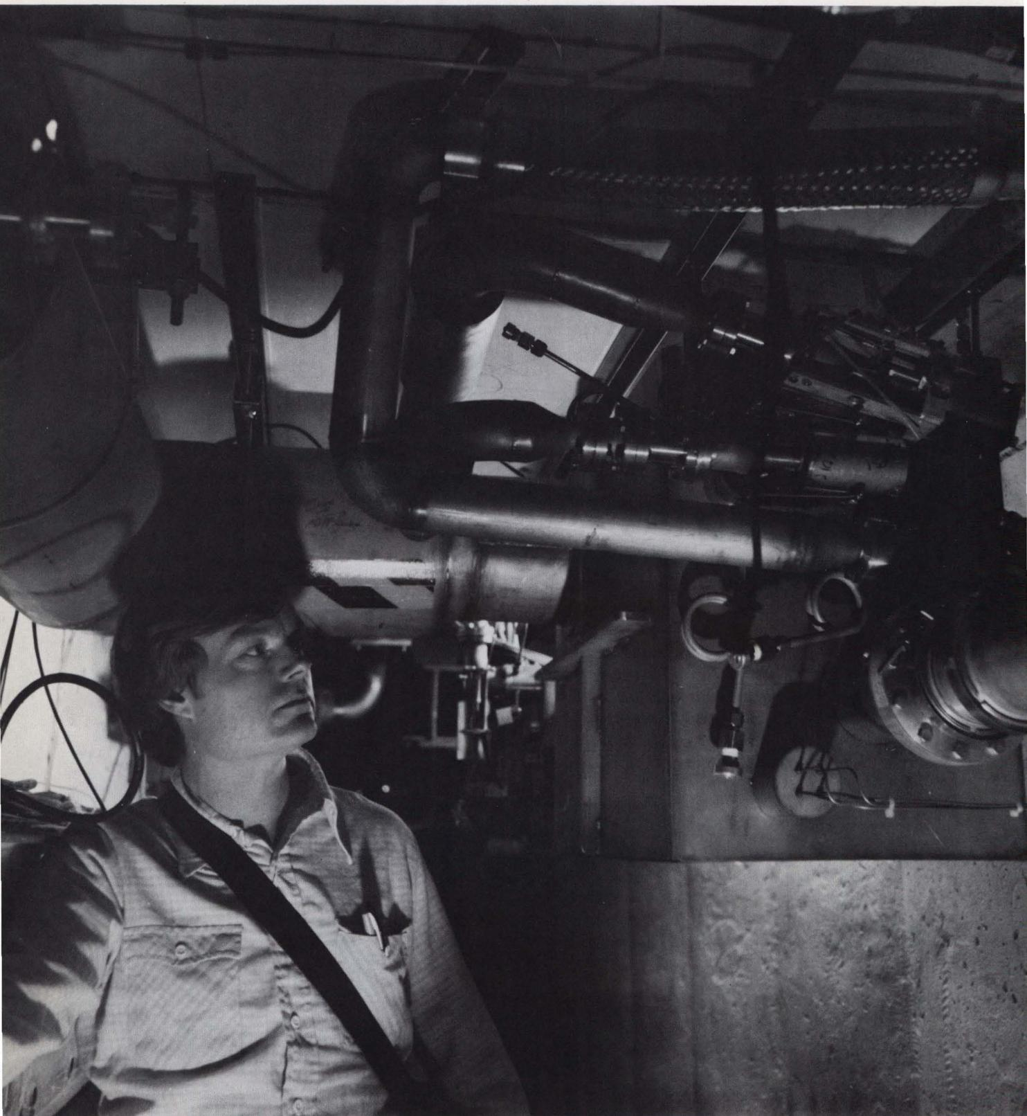
Roger Dixon inspects the installation of the superconducting beam line in the Switchyard.
