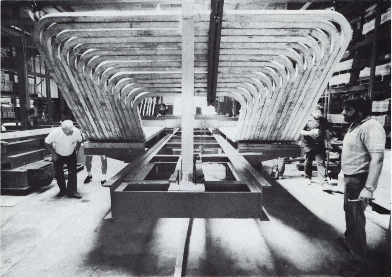
Les Bradstreet (left) and John Chyllo check positioning of the pancake coil moved into Industrial Building 4 to be off-loaded onto the assembly fixture.
