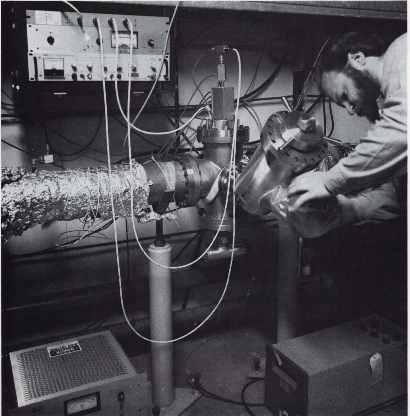
Don Poll works on the vacuum system of the Electron Cooling Ring.
