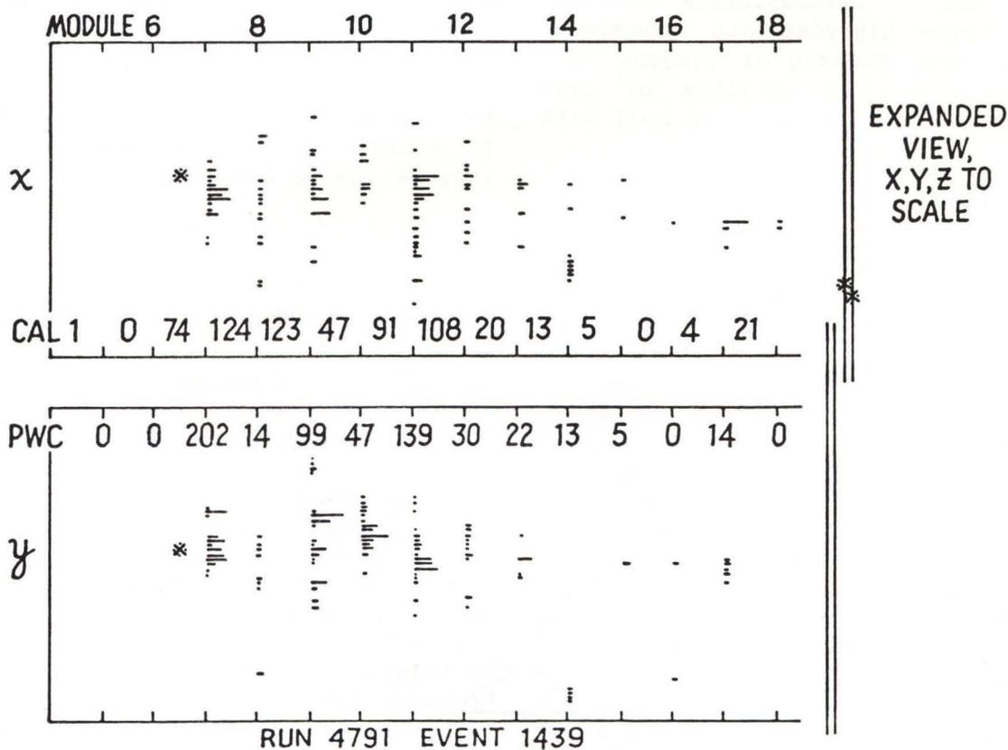
A typical  $\nu_\mu$  charged-current interaction in E-613. The visible hadronic energy is 168 GeV. In the expanded view, the calorimeter and proportional wire chamber energy depositions are expressed in terms of numbers of equivalent muons.
