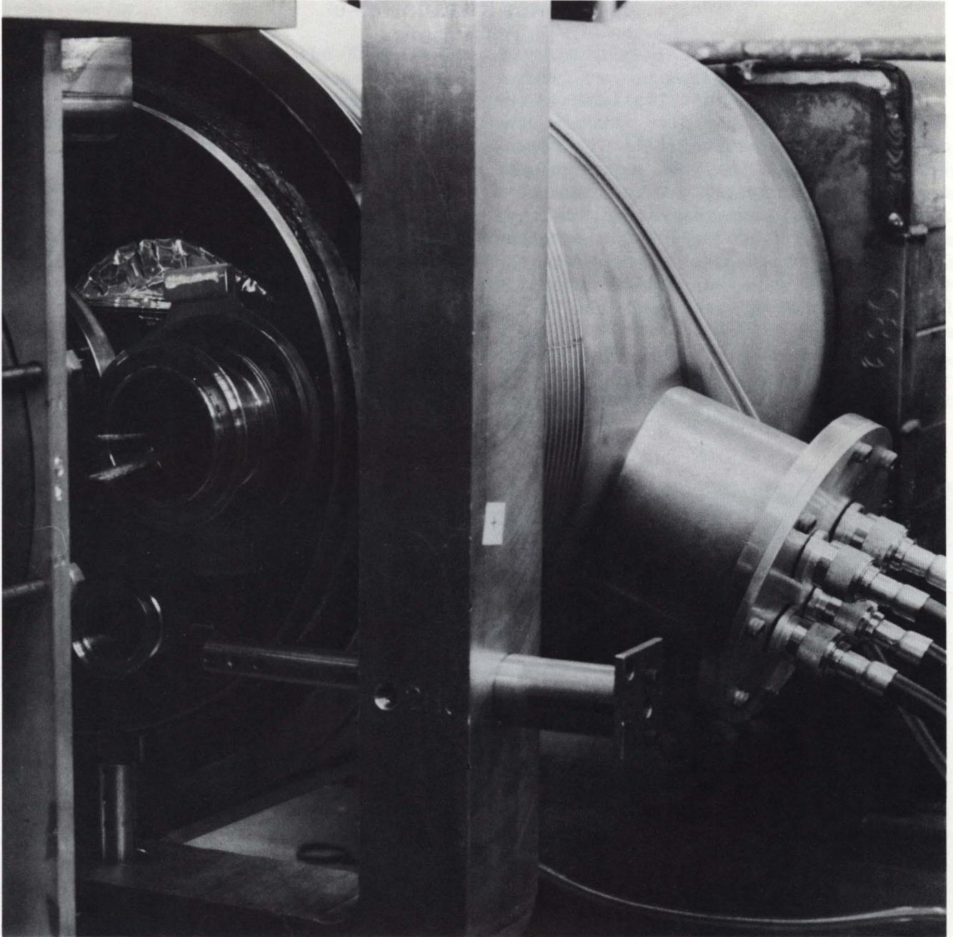
The location of a beam-position detector next to a quadrupole. The cables at the right are the leads to the detector, which was developed by Bob Shafer.
