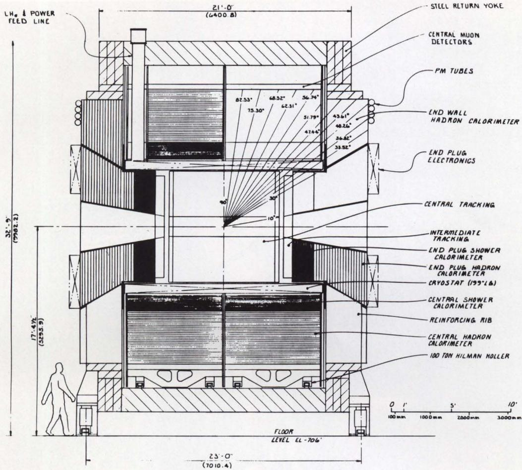
A side view of the details of the Collider Detector.
