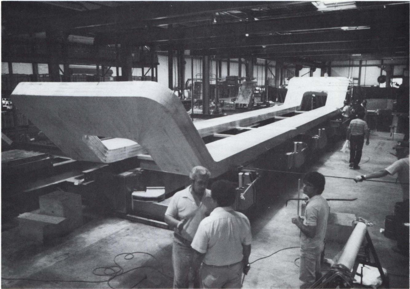
Foreground (left to right) Dominic Carullo, Isidro Gonzales, and Oscar Guerra check installation of a four-layer coil onto the Meson assembly fixture.
