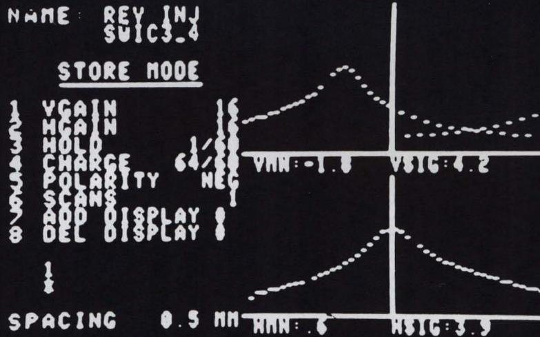
Beam signals from 80-GeV protons extracted from the Main Ring at F17 for antiproton production. The upper trace shows the vertical distribution, the lower trace the horizontal.
