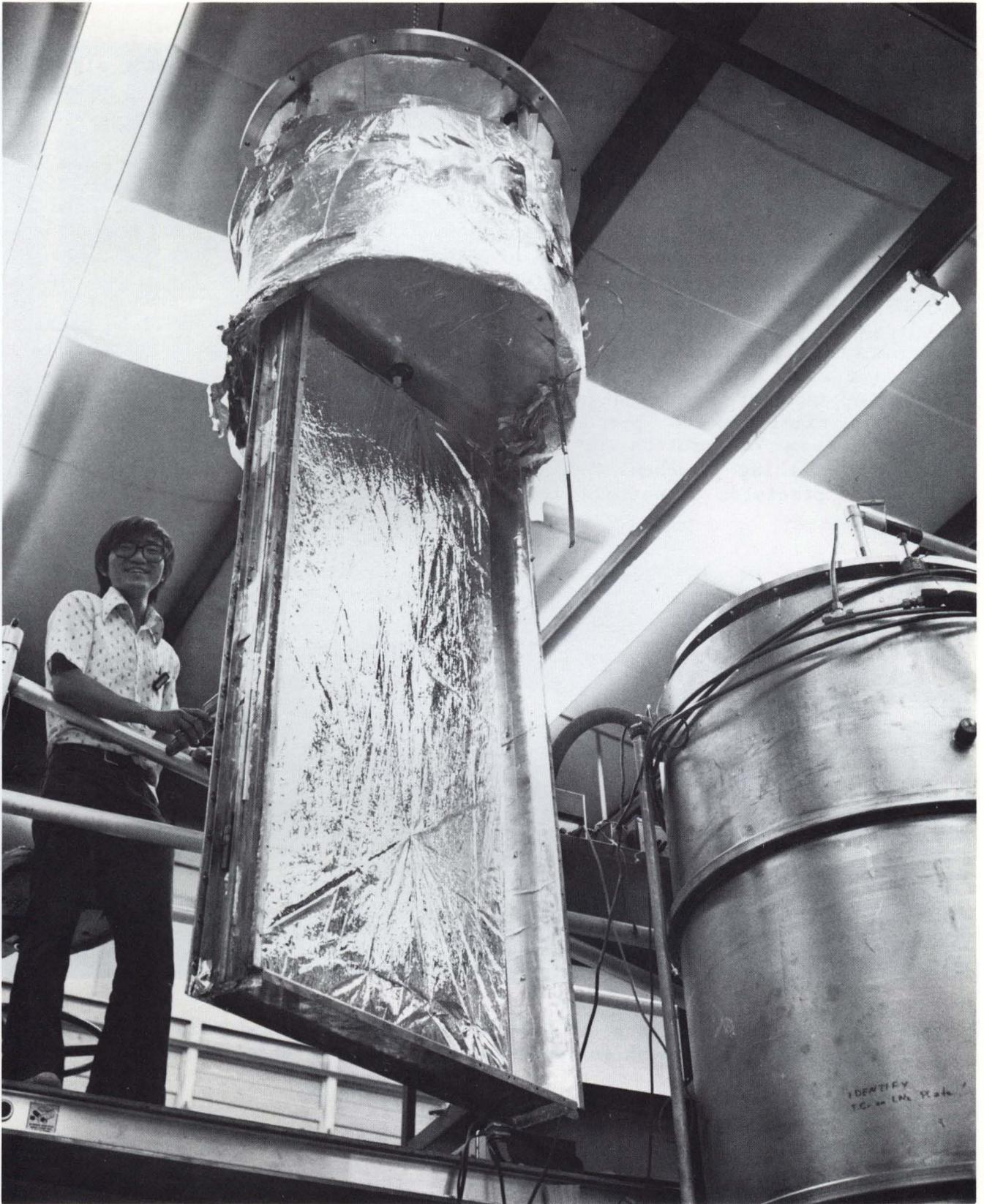
Eddie Leung with a partially disassembled helium dewar to reduce heat loss.
