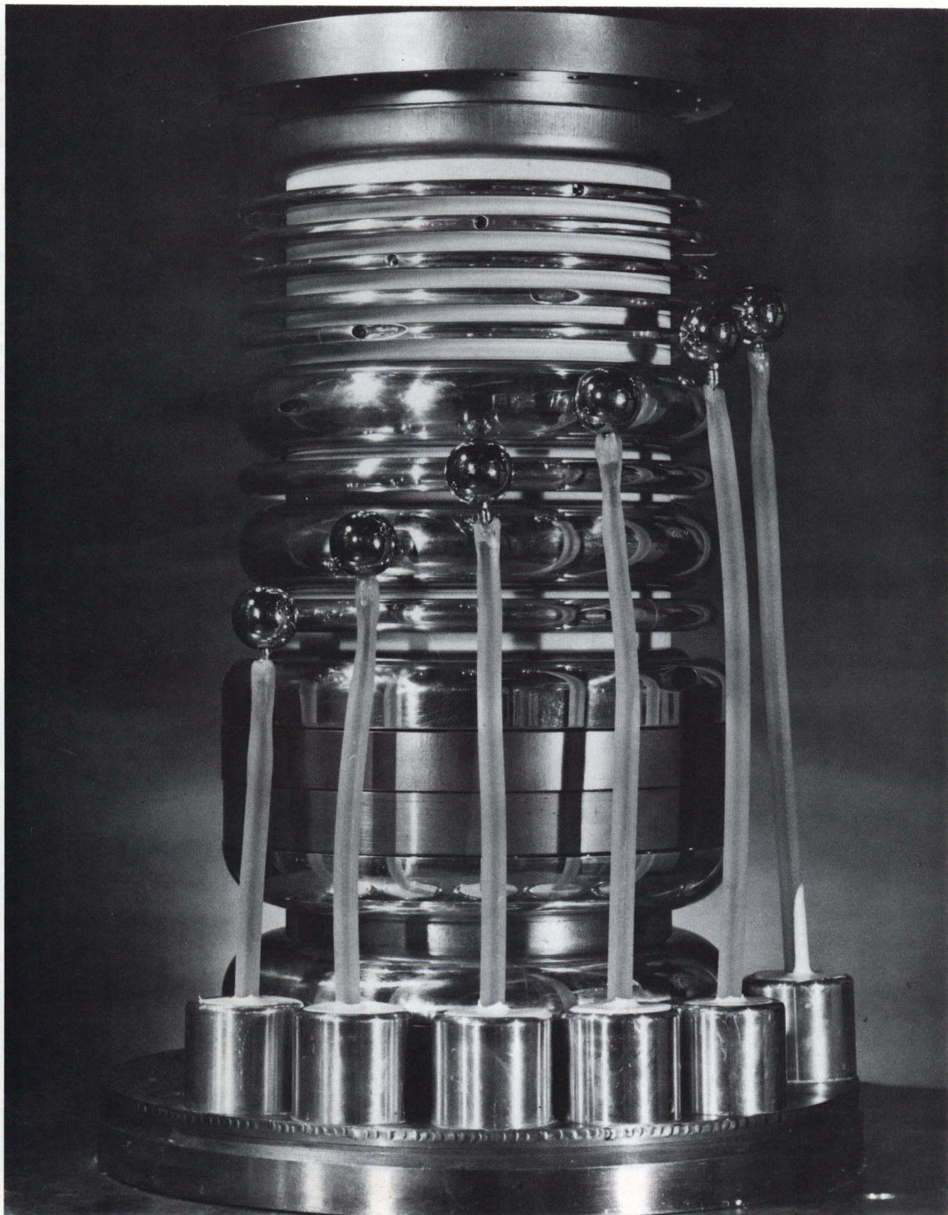
The accelerating column of the electron gun system for the Electron Cooling Ring.
