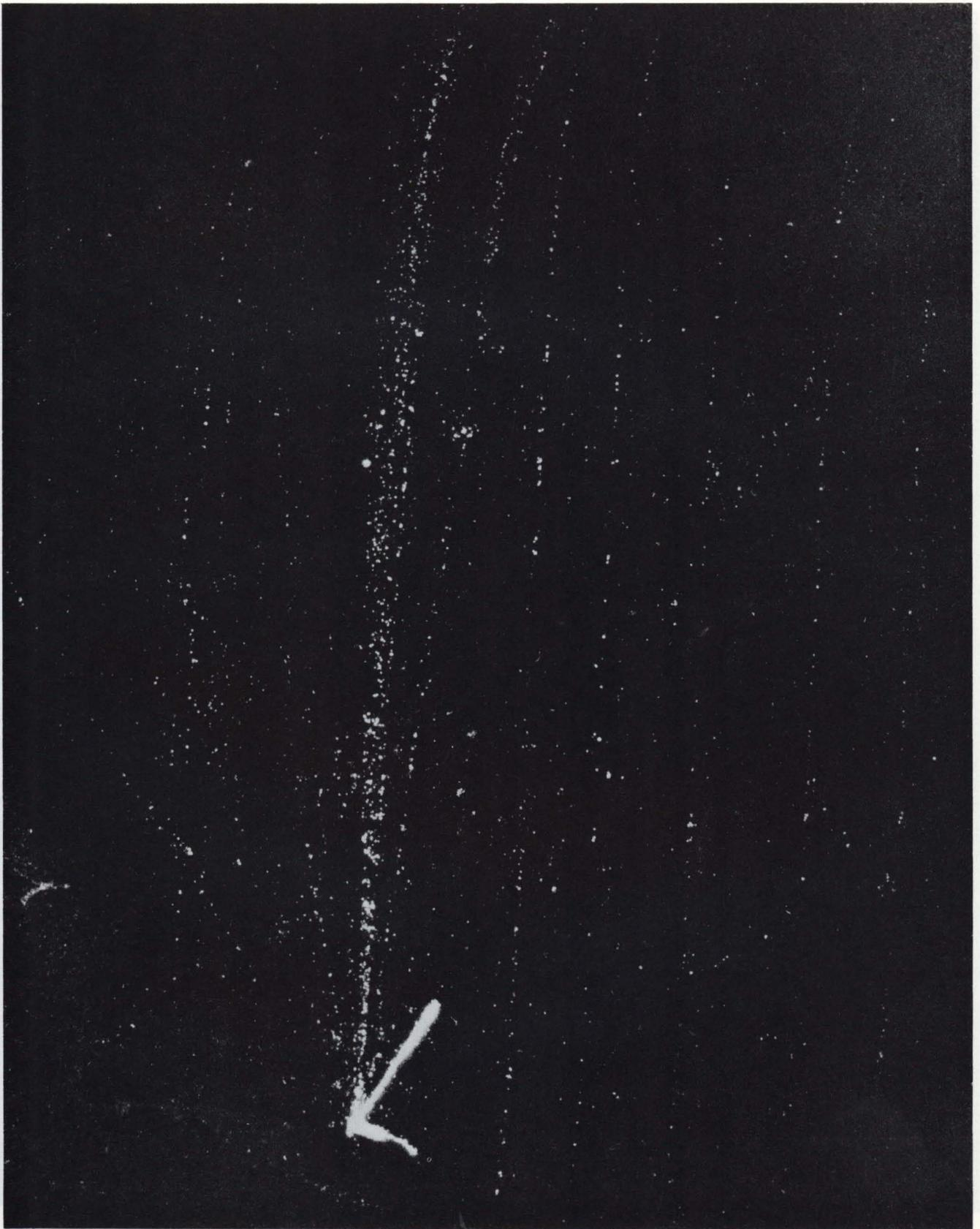
Interaction of a 200-GeV pion in the sodium-iodide scintillation camera of E-515. The 10-micron resolution of this system will permit direct observation of charmed-particle decays.
