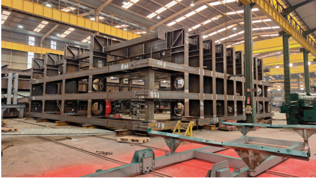
Figure 5: The pre-assembly of a section of the second cryostat for the DUNE far detector at the factory in Arteixo, Spain. Credit: CERN.
