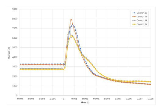
The magnet was protected by a 60 m $\Omega$  dump resistor to extract the stored energy
