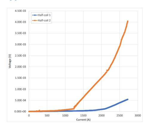
The half-coil 2 that limited the magnet performance also showed a much larger voltage than the half-coil 1
