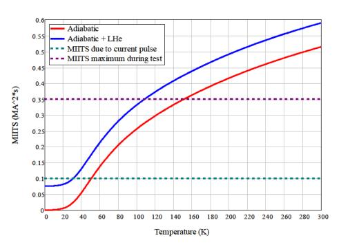
Due to the small cross-section area of the stabilizer (only 1.42 mm<sup>2</sup> per conductor), the magnet reaches high temperatures at a low number of MIITS
