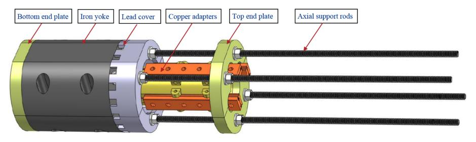
60 mm clear bore, 80 mm coil OD, two half-coils made with two layers of round STAR® wire The non-insulated conductor is wound into a continuous channel in the insulating (ULTEM) structures The leads are terminated at 3 copper adapters that allows to test each coil individually Redundant voltage taps co-wound with the conductor into the support structure
