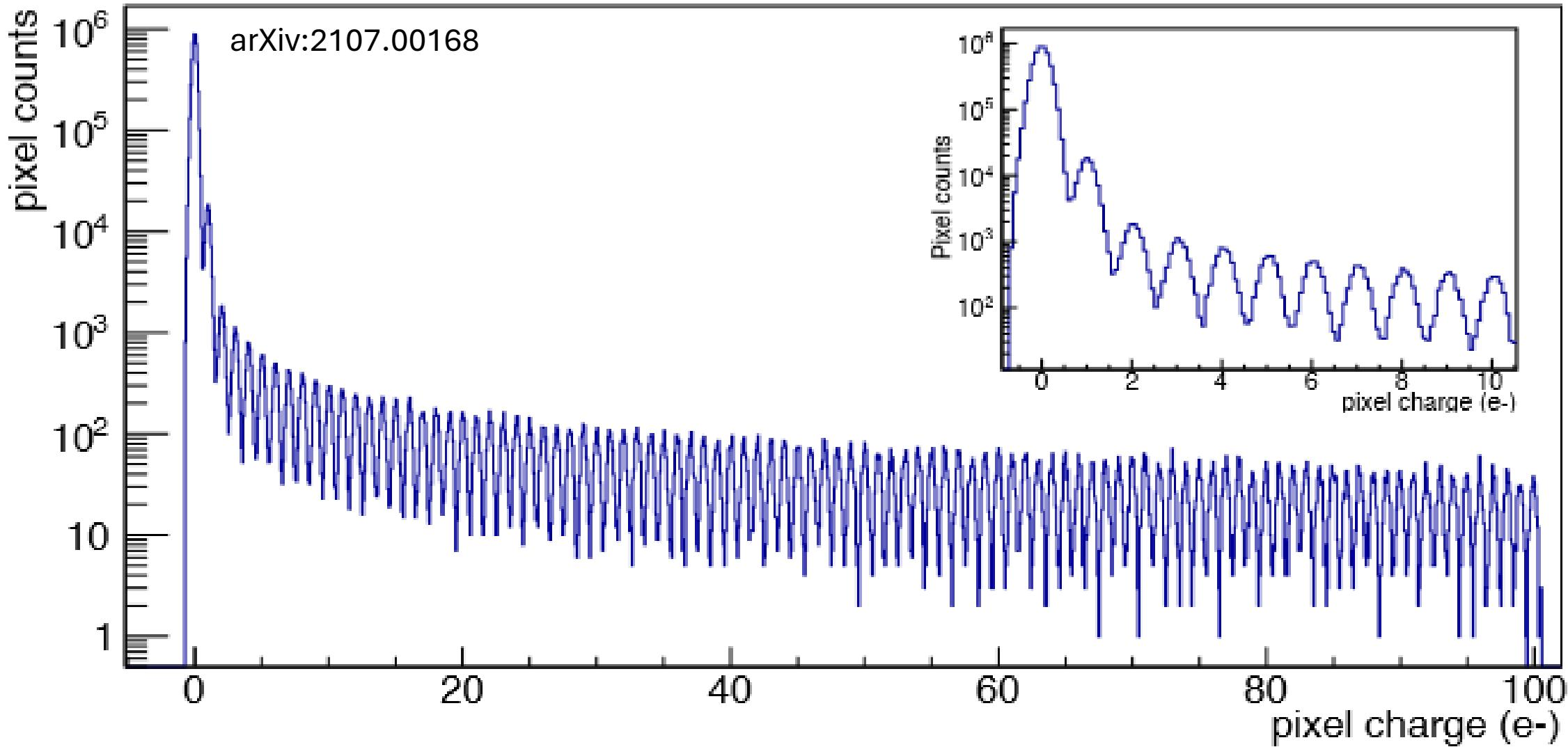
Photon counting allows direct gain measurements at low and high signal levels
