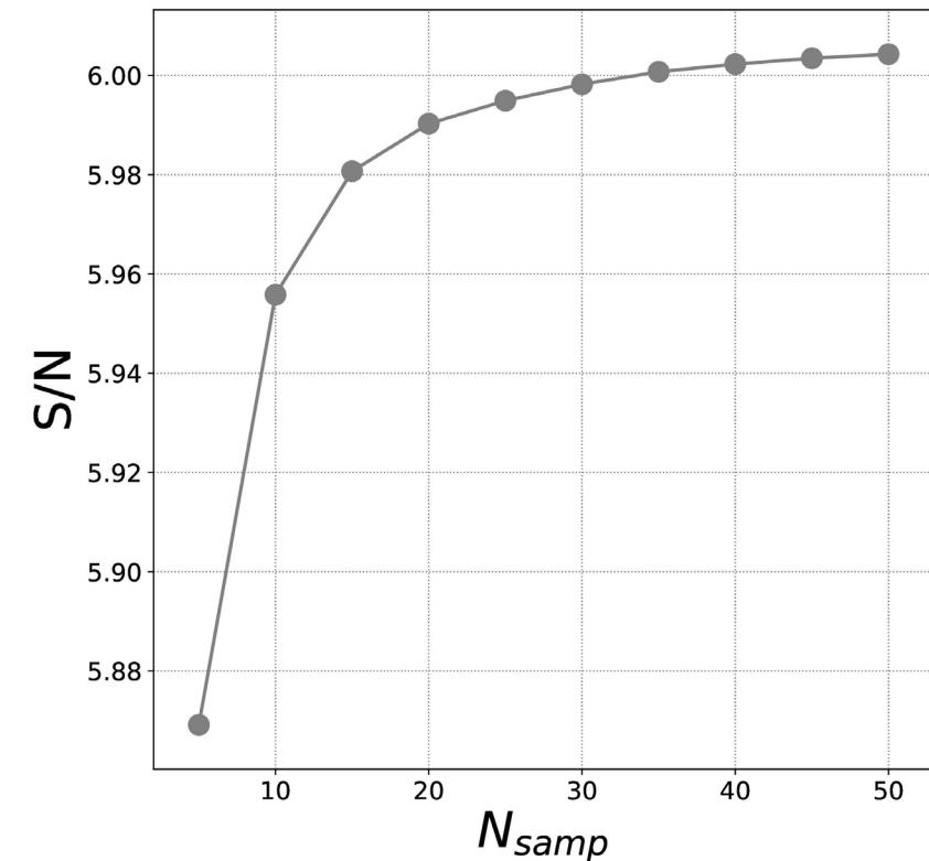
Skipper CCDs retain the performance of conventional CCDs at high signal-levels. Improvements to the signa-to-noise only in the readout noise dominated regime.
