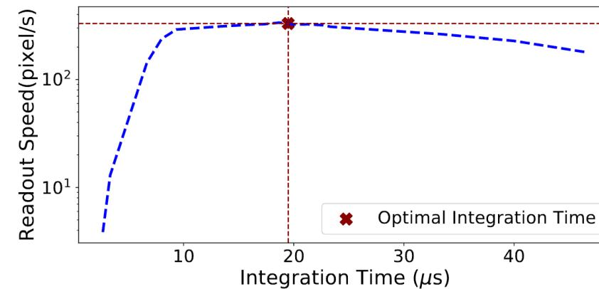
Optimize for pixel integration time and number of samples per pixel to reach target noise the fastest
