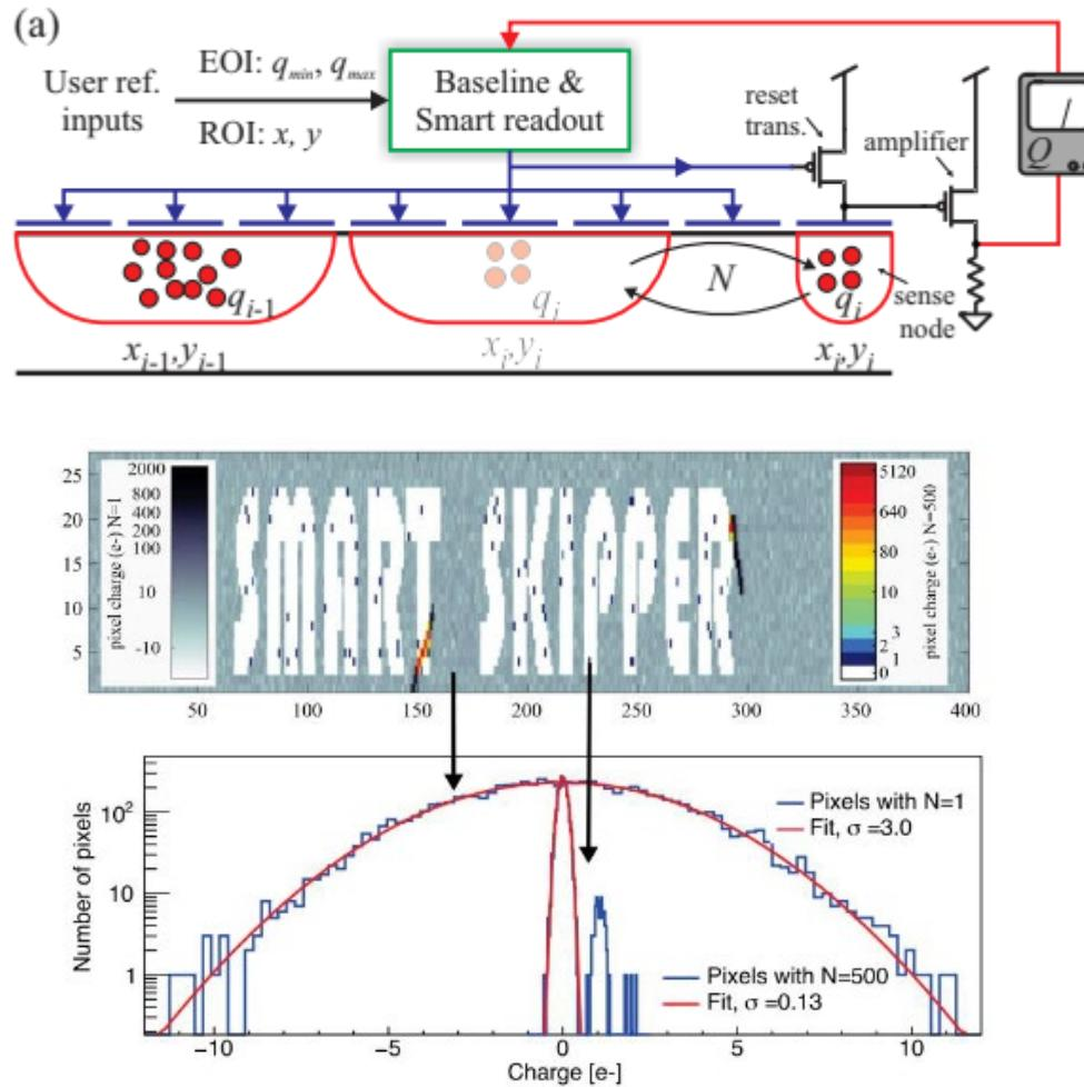
FIG. 3. Measurement using ROI technique. Pixels in the words have  $N = 500$  (right scale); pixels outside the words have  $N = 1$  (left scale).  $s_f$  was zero in most pixels, with some pixels having  $s_f = 1, 2, 3$  or very large values for the two muon tracks that are observed.
