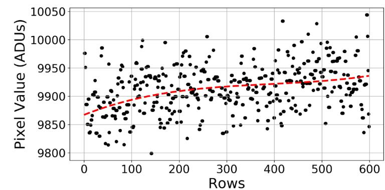
Median filter and spline fit row-by-row in single- and multi-sample serial overscan regions
