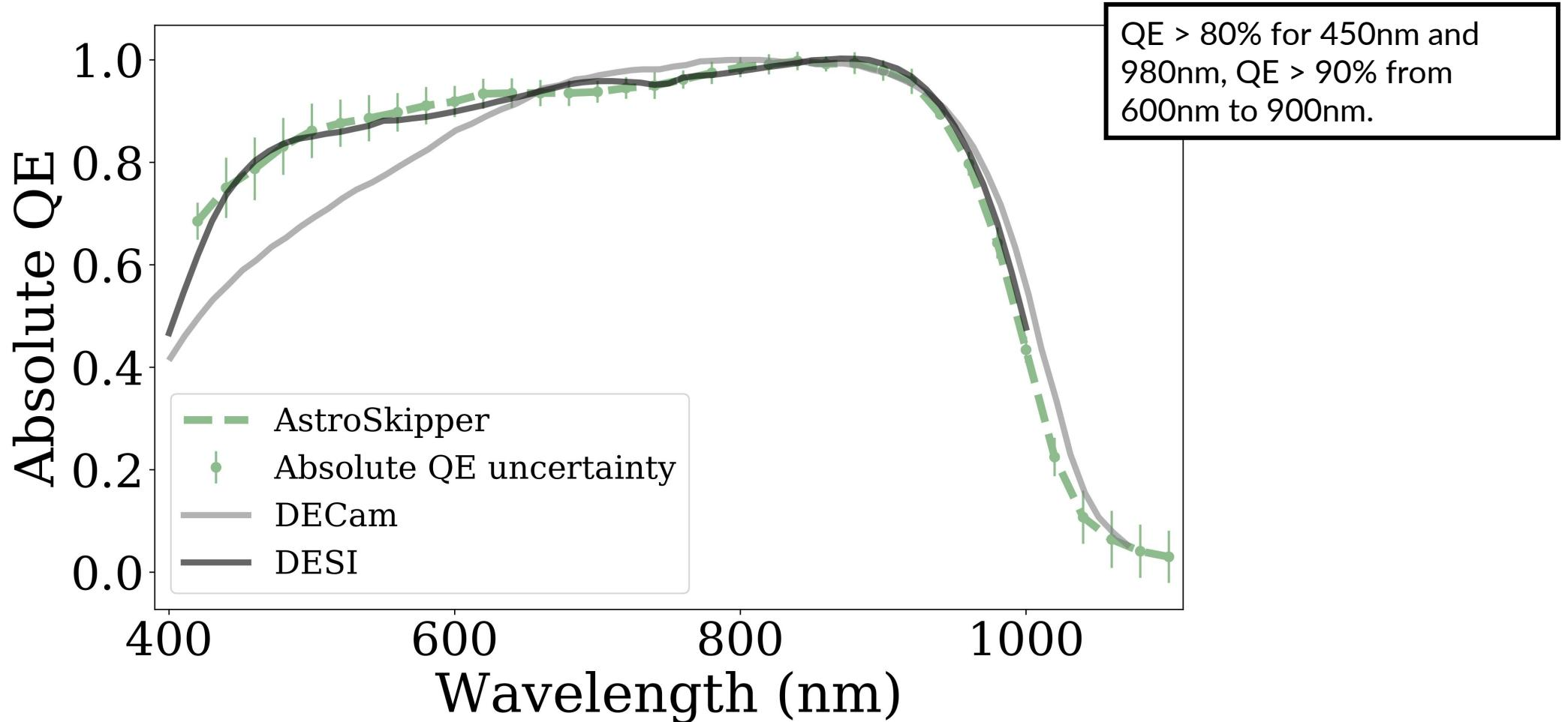
AstroSkippers retain the high QE of the thick, fully depleted DESI detectors from LBNL
