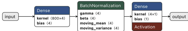
FIG. 4. Visualization of a two-layer neural network architecture with an 800-dimensional input, a dense layer with batch normalization followed by another dense layer with a sigmoid activation function.
