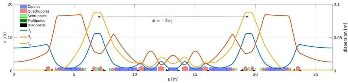
**Fig. 1** Lattice functions and magnets layout for the HMBA SR standard cell with two symmetric CCS. Horizontal and vertical steerers and skew quadrupoles are located in each corrector and sextupole depicted in the layout. The  $\beta_x$ ,  $\beta_z$ , and  $\eta_x$  Twiss parameters are shown as blue, red, and orange lines, respectively. Reproduced from Ref. [10] under Creative Commons License 4.0 (<https://creativecommons.org/licenses/by/4.0/>)
