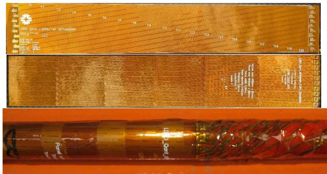
**Fig. 2.** Top two: Flex-QA used in magnet testing – two types of QA are employed; Bottom: quench antenna panels wrapped precisely around their support (270 mm diameter, visualized on Fig.1).
