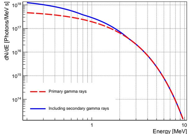
FIG. 3. Photon flux produced in the nuclear reactor. The red dashed line is derived from Eq. 1, considering primary  $\gamma$ -rays only. The blue solid line is obtained from a GEANT4 simulation, taking into account secondary photon production.
