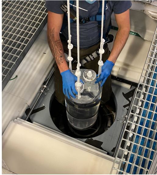
Figure 21: Deployment of the GdLS plug – a small cylindrical acrylic tank with neutral buoyancy. It is used to fill the cut-out during the science run and is only replaced with the YBe source during calibrations.
