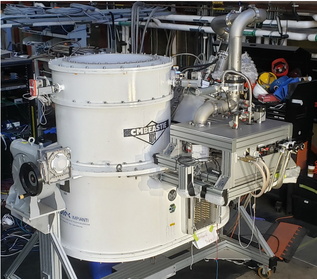
Figure 3. The fully assembled SAT-MF1 in the UC San Diego laboratory space. The rack mounted to the side houses the turbomolecular pumps for the DR circuit and is attached to the receiver with a mounting jig for testing.
