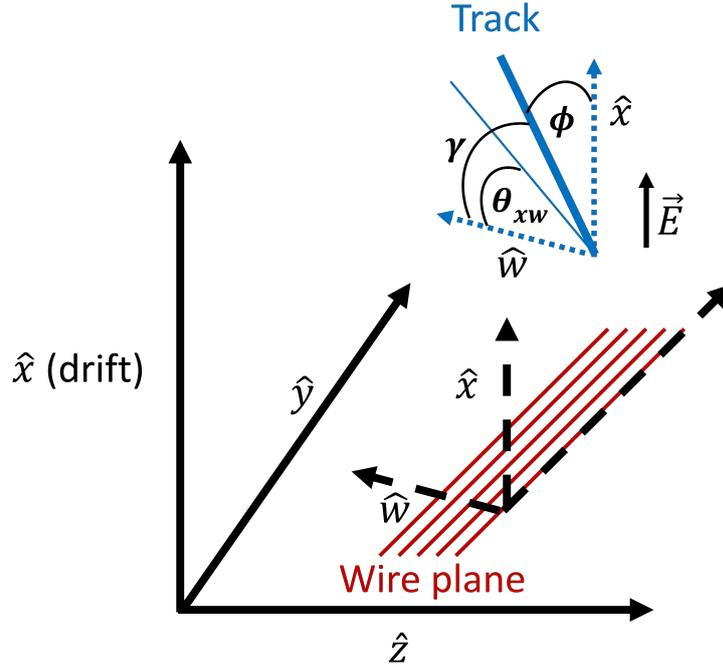
**Figure 2.** Diagram of relevant track angles.  $\gamma$ , the angle of the the track to the direction perpendicular to the wire direction, determines the track pitch.  $\phi$ , the angle of the track to the drift electric field, controls any angular dependence in electron-ion recombination.  $\theta_{xw}$ , the angle of the track between the drift electric field direction and the direction perpendicular to the wire direction, controls the track ionization signal shape.
