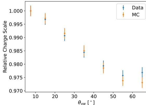
**Figure 4.** Relative scale of charge reconstruction as a function of the track angle  $\theta_{xw}$  (see figure 2), determined in ICARUS data and Monte Carlo simulation. A systematic uncertainty of 0.2% on the correction is assigned to cover the difference between data and Monte Carlo simulation.
