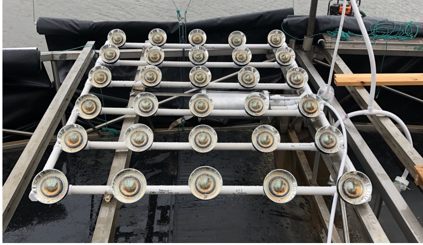
Figure 15: Completed Nikhef plane installed in the detector. Each PMT has an acrylic cover and reflector attached. The PMTs are sealed inside their inserts and installed into the PVC plane frame. The electronics container located in the centre of the plane. A flexible PVC hose (incomplete) exits the electronics container, which would connect the plane to upstream power supplies and DAQ electronics.
