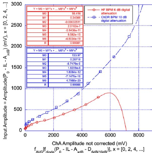
Figure 5: Plot of the input signal amplitude from the pulse generator against the amplitude reading (not corrected) of ChA for both the HF BPM electronics and the ChDR BPM electronics.
