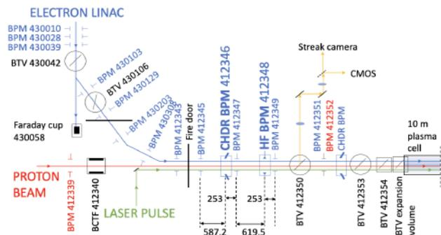
Figure 2: Schematic of the common beamline at AWAKE indicating the beam instruments.
