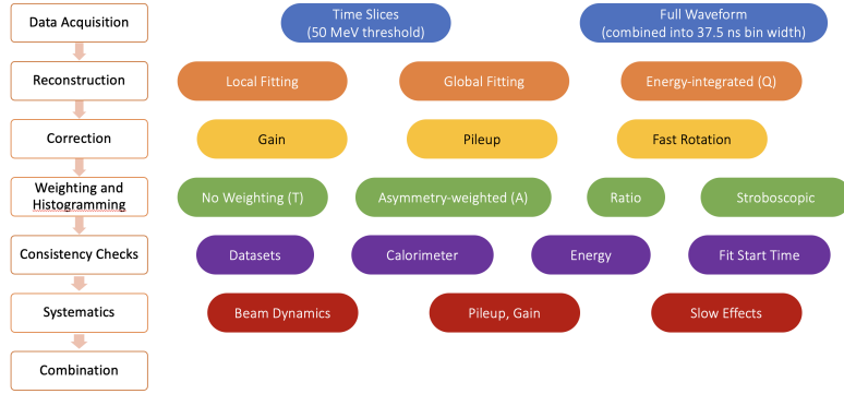
Figure 3: Analysis flow for \omega_a extraction and systematics assessment. The process integrates raw data modeling, beam dynamics corrections, and iterative systematic studies to ensure the accuracy and reliability of the extracted precession frequency.
