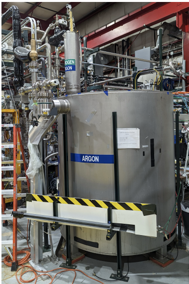
FIG. 2. The ICEBERG cryostat. One of two scintillator bars for cosmic triggering is visible at the front bottom of the cryostat.
