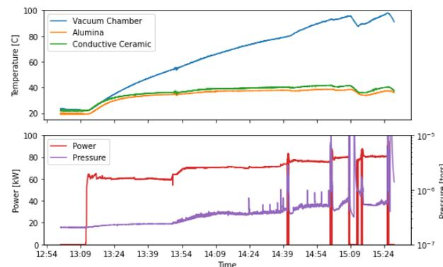
Figure 3: Temperature, power, and pressure vs. time for the second field configuration during the 650 MHz high power test.
