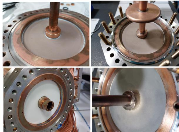
Figure 6: Photos of the conductive ceramic (top) and alumina (bottom) windows, before (left) and after (right) the high power test.
