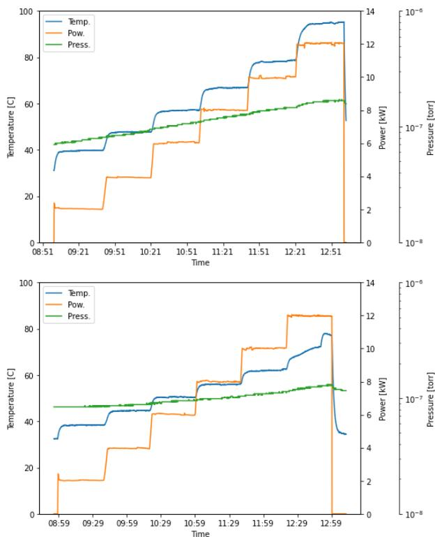
Figure 1: RF power (orange), window temperature (blue), and pressure (green) vs. time for each window during the 1.3 GHz high power test.
