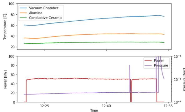
Figure 5: Temperature, power, and pressure vs. time for the fourth field configuration during the 650 MHz high power test.
