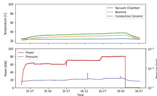
Figure 2: Temperature, power, and pressure vs. time for the first field configuration during the 650 MHz high power test.
