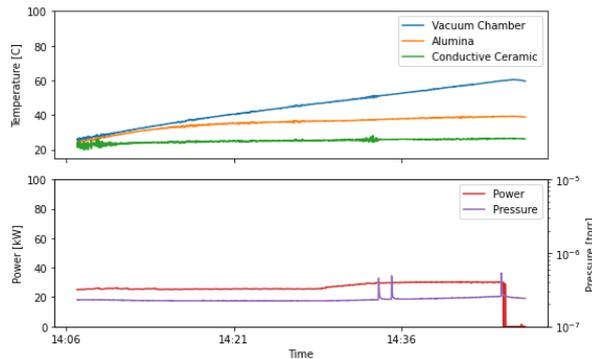
Figure 4: Temperature, power, and pressure vs. time for the third field configuration during the 650 MHz high power test.
