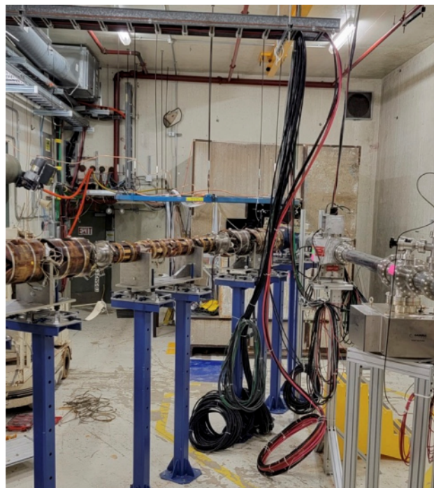
Figure 1: Low-energy pion/muon beamline recently installed at Fermilab MeV Test Area.
