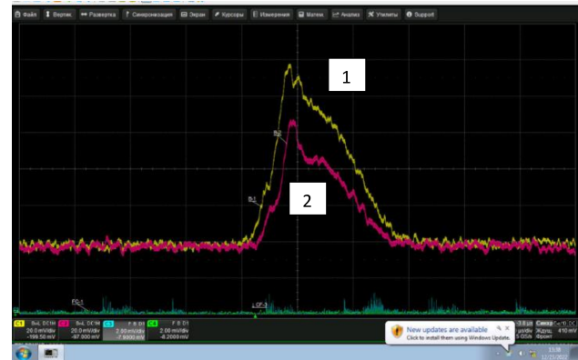
Figure1: Signals of current transformers at the RFQ exit (curve 1) and the HILAC exit (curve 2).
