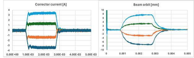
Figure 4: Measured beam position with applying +/- 3.4 A and +/- 1.63 A on the corrector.
