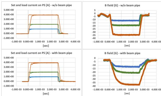
Figure 3: Set and load current on corrector power supply (left). Measured magnetic field (right). Top: without beam pipe, Bottom: with beam pipe.
