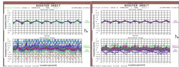
Figure 8: Beam orbit jitter without (left) and with (right) the amplitude compensation using corrector dipole.
