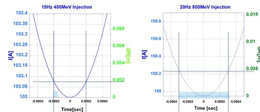
Figure 1: GMPS current and radial position shift with constant RF frequency. Left: Present 15 Hz operation, Right: PIP-II 20 Hz operation.
