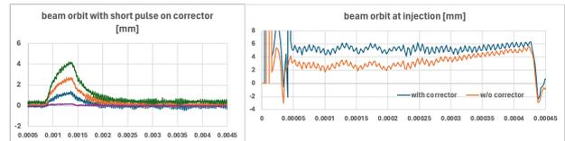
Figure 5: Left: Beam orbit with shorter pulse on corrector. Right: Effective bending field flattening with corrector. Beam position with correction (blue) without correction (orange).
