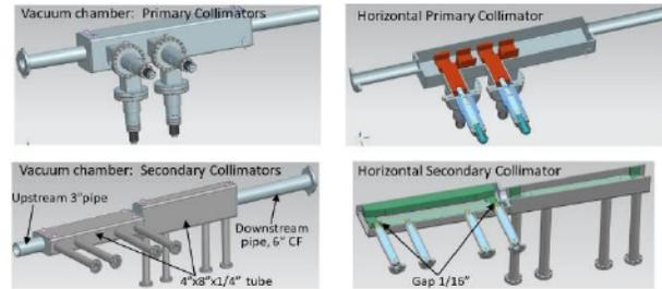
Figure 6: Primary and secondary collimator vacuum chambers with collimator jaws.
