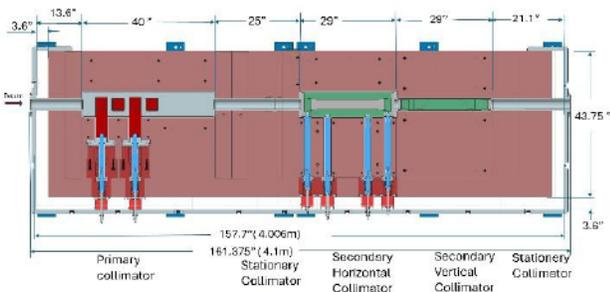
Figure 3: Plan view cross section of the 2SC unit showing the horizontal primary and secondary jaws.
