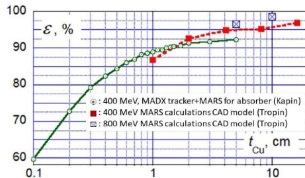
Figure 1: Collimation efficiency  $\varepsilon$  vs the primary copper jaw thickness  $t_{Cu}$ .
