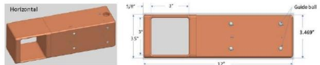
Figure 5: 3D and plan view of the primary horizontal copper collimator. The vertical primary has the same design features.
