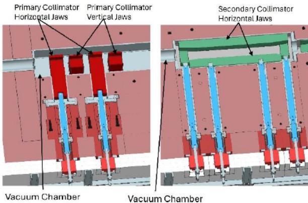
Figure 4: Horizontal sectional view of primary and secondary collimator jaws bisected in beam plane.
