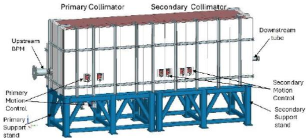
Figure 2: CAD drawing of the 2SC to be installed in the Booster tunnel.
