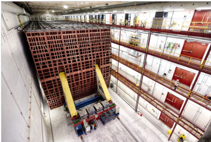
Far Detector 15.5m x 15.5m x 60 m surface
