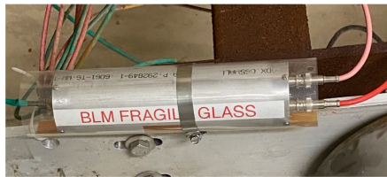
Beam Loss Monitor
