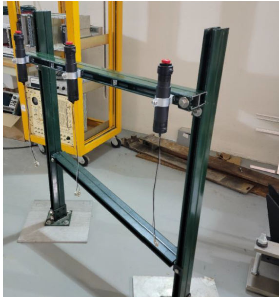
Figure 2.5: The three PMTs are installed on the arm prior to installation.
