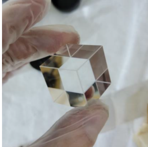
Figure 2.3: One of the quartz crystals that'll be used as the signal source for the PMT.
