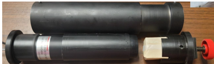
Figure 2.4: The PMT assembly depicting the cylindrical housing at the top, PMT with end-cap in the bottom left, and quartz crystal in the holder on the bottom right.
