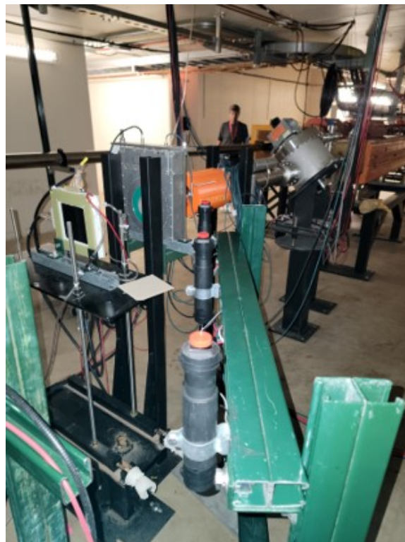
Figure 1.8: The real setup showing the target position with respect to the angled telescope detector setup.
