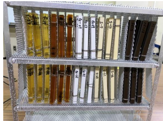
Fig. 7. Picture of aluminum crate containing the resins to be gamma ray irradiated in air atmosphere.
