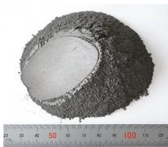
Fig. 2. Micrograph of the HoCu 2 particles produced by a standard melt and casting process.
