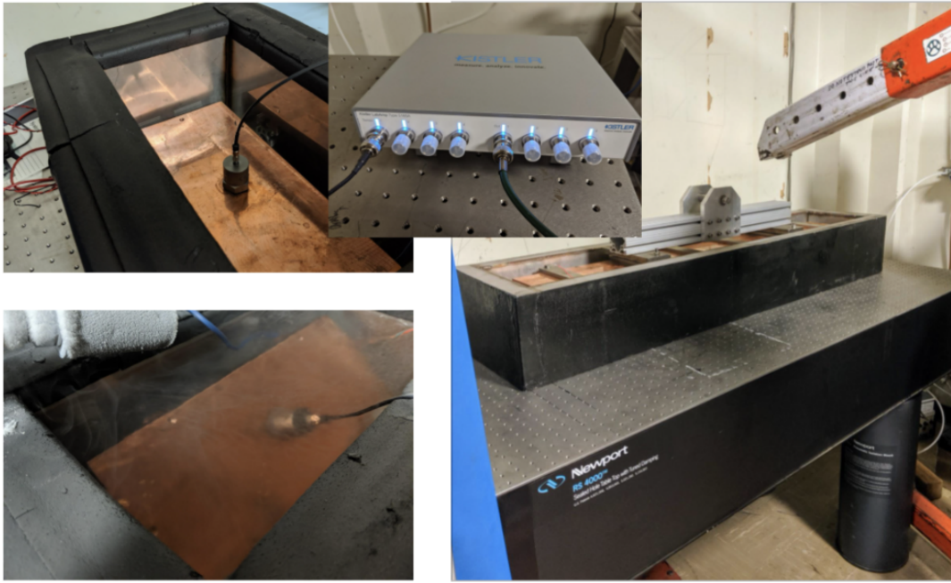
Figure 22. Test bed for measuring vibrations from the boiling of liquid nitrogen due to applied thermal load in copper structure.
