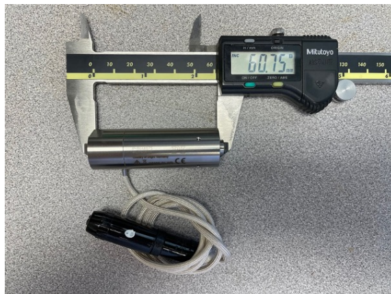
Figure 21. A 200 micron travel piezoelectric actuator. Actuators operate at cryogenic temperatures and high mechanical loading. The devices were developed for LCLS-II.
