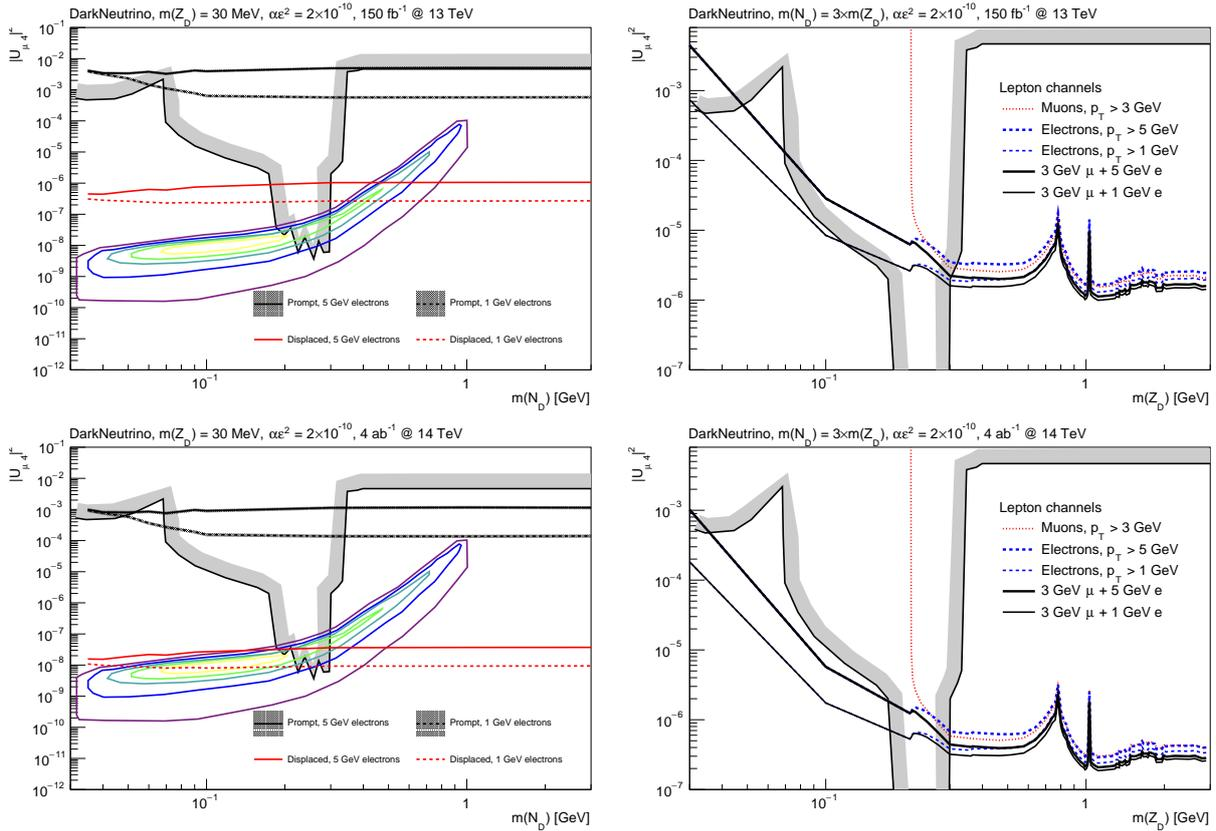
FIG. 9: Expected upper limit on the neutrino mixing parameter  $U_{\mu 4}$  are shown as a function of the  $Z_D$  mass for several assumptions about the classes of potentially reconstructable leptons. Comparisons are made for the Run 2 (top row) and HL-LHC data sets (bottom row), and for the  $m_{Z_D} = 30$  MeV (left column) and  $m_{N_D} = 3m_{Z_D}$  (right column).
