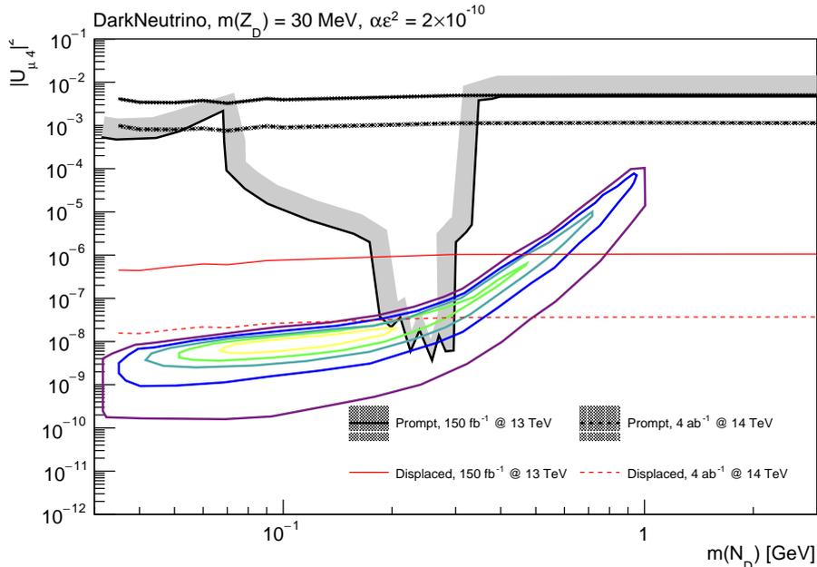
FIG. 6: The ranges of neutrino mixing parameters expected to be excluded by LHC experiments during Run 2 and the HL-LHC are shown versus  $N_D$  mass for a fixed  $Z_D$  mass of 30 MeV. Upper limits on  $U_{\mu 4}$  are shown for both the prompt and displaced search strategies, with uncertainty bands described in the text. Closed contours correspond to the parameters favored by Ref. [10] at the 1, 2, 3, 4 and 5-sigma confidence level.
