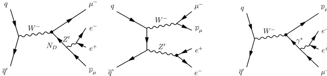
FIG. 1: Representative diagrams are shown for the production of  $e^+e^-$  pairs from dark photon decays in  $W^- \rightarrow \mu^- \bar{\nu}_\mu$  events, produced either through the mixing of neutral leptons (left) or  $U(1)$  gauge forces (center). At right the dominant SM background process is shown, in which the muon radiates an  $e^+e^-$  pair via virtual photon emission.
