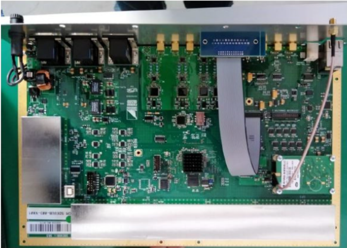
Figure 7. Assembled UUB, equipped with front panel, GPS receiver, cables and shielding covers.
