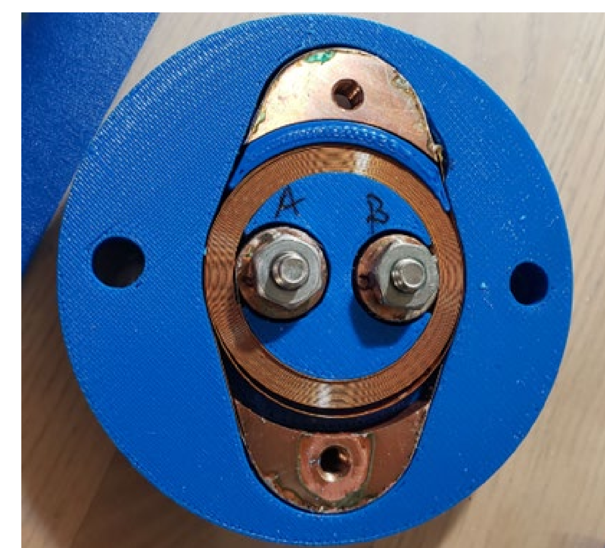
Small REBCO coil fabricated from 4mm tape with IC of \sim 95 A at 77 K
