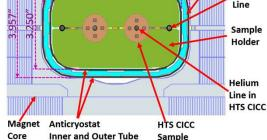
The Sample Cable Holder shares similarities with the EDIPO sample holder, featuring a rectangular shape reminiscent of a magnet. Its purpose is to precisely position the cable, aligning it with the desired spacing and orientation within the magnetic field.
