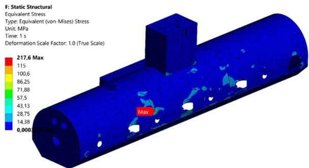
Figure 8: Stress of the thermal shield during the cooling down with a cooling down rate of 20 K.h<sup>-1</sup>.
