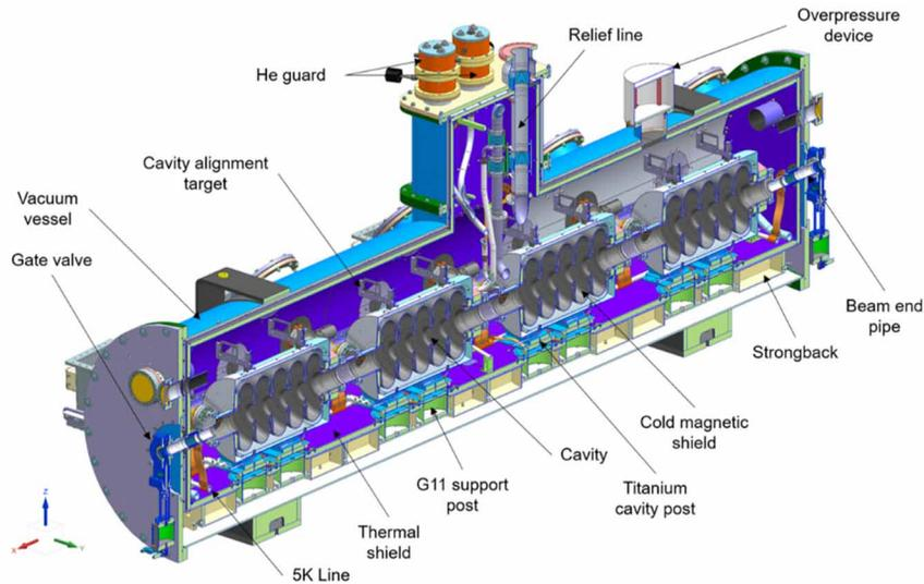
Figure 2: Layout of the LB650 cryomodule.
