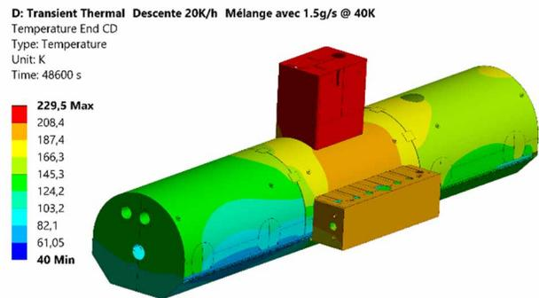
Figure 7: Temperature distribution of the thermal shield 13.5 h after the start of the cool down, with a cooling down rate of 20 K.h<sup>-1</sup>.
