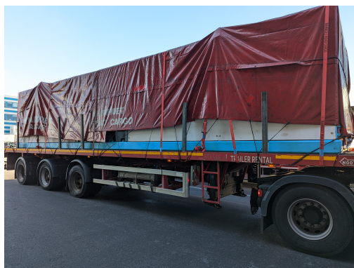
Figure 8: Tarping of the frame in two parts by vendor at LUX airport.
