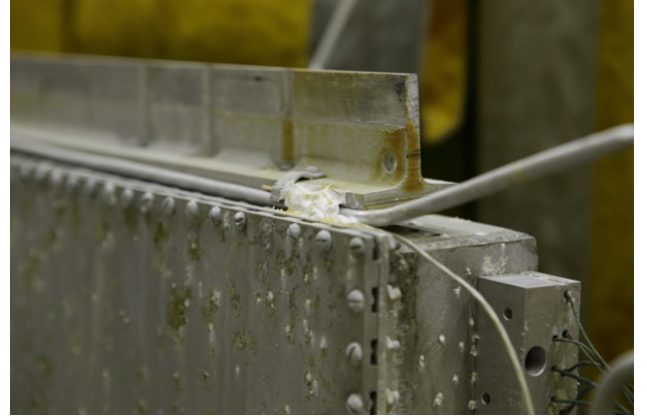
Figure 8: Picture shows the upper right of the hadron monitor which used in the NuMI beamline for a couple of years.
