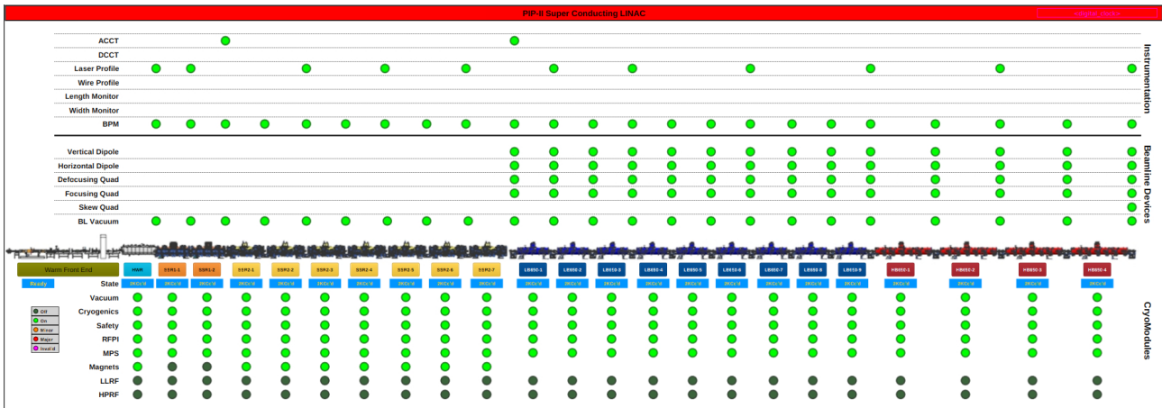
Figure 6: Prototype operator main page for PIP-II accelerator [1].
