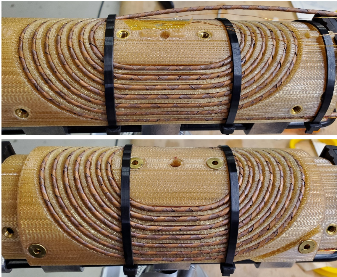
Figure 7. Inner (top) and outer (bottom) layers of half-coil 1 as wound.
