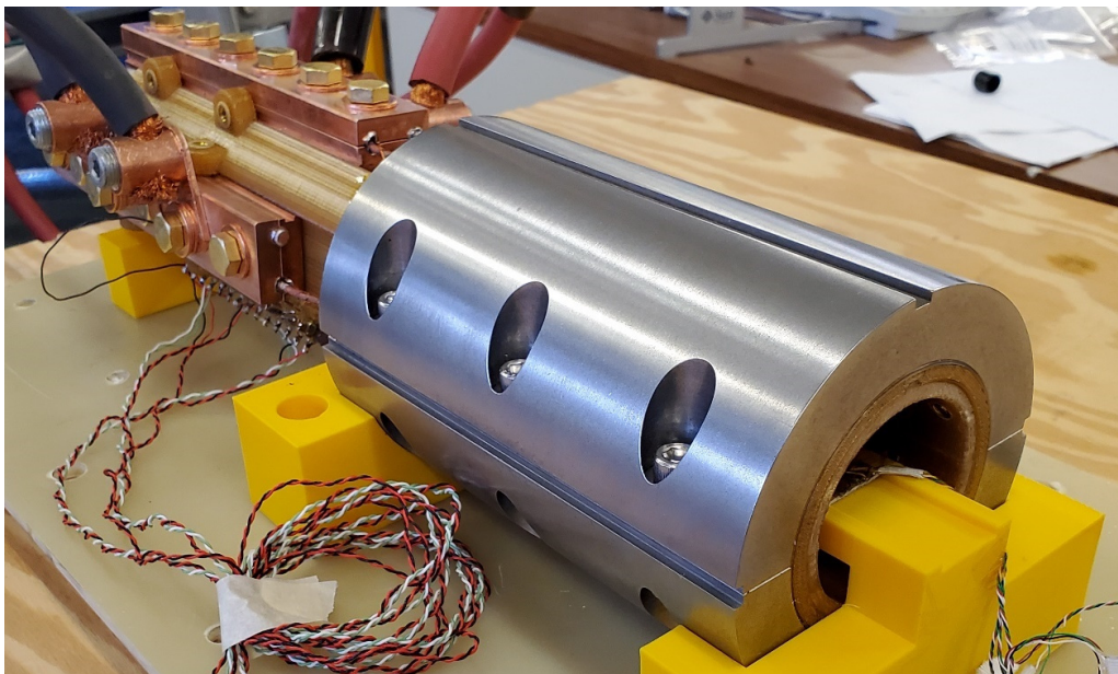
Figure 8. Two half-coils assembled with the lead support and the ground insulation (top) and the magnet with the power leads attached prior to testing in liquid nitrogen (bottom).
