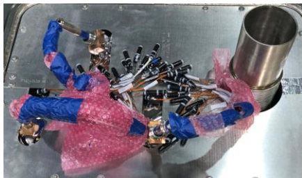
Figure 7: Wires through the pressure transducer lines.
